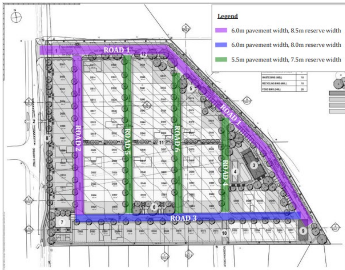
Figure 31. Internal Road Network Hierarchy (Source: InRoads Group, 2025)
