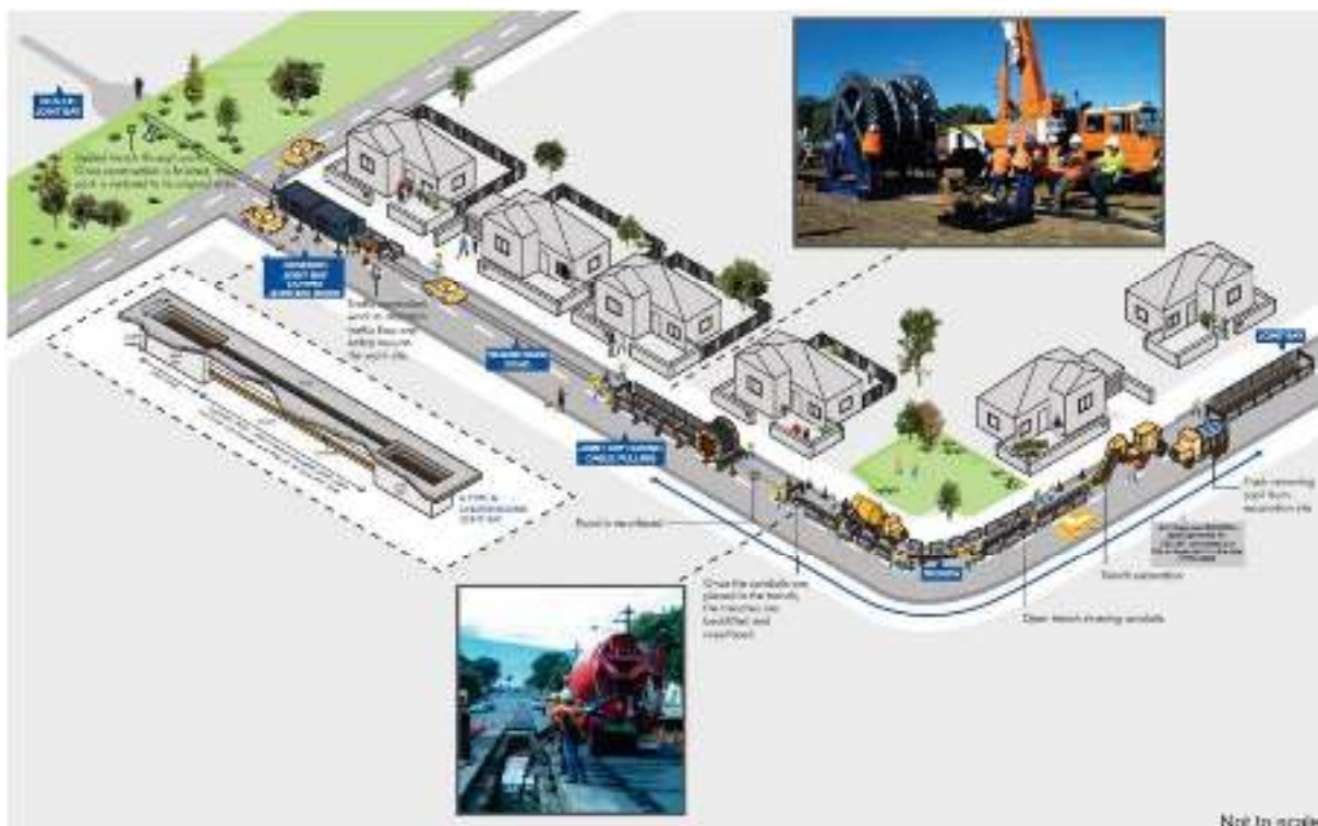
Figure 3; TransGrid indicative overview of typical construction activities
