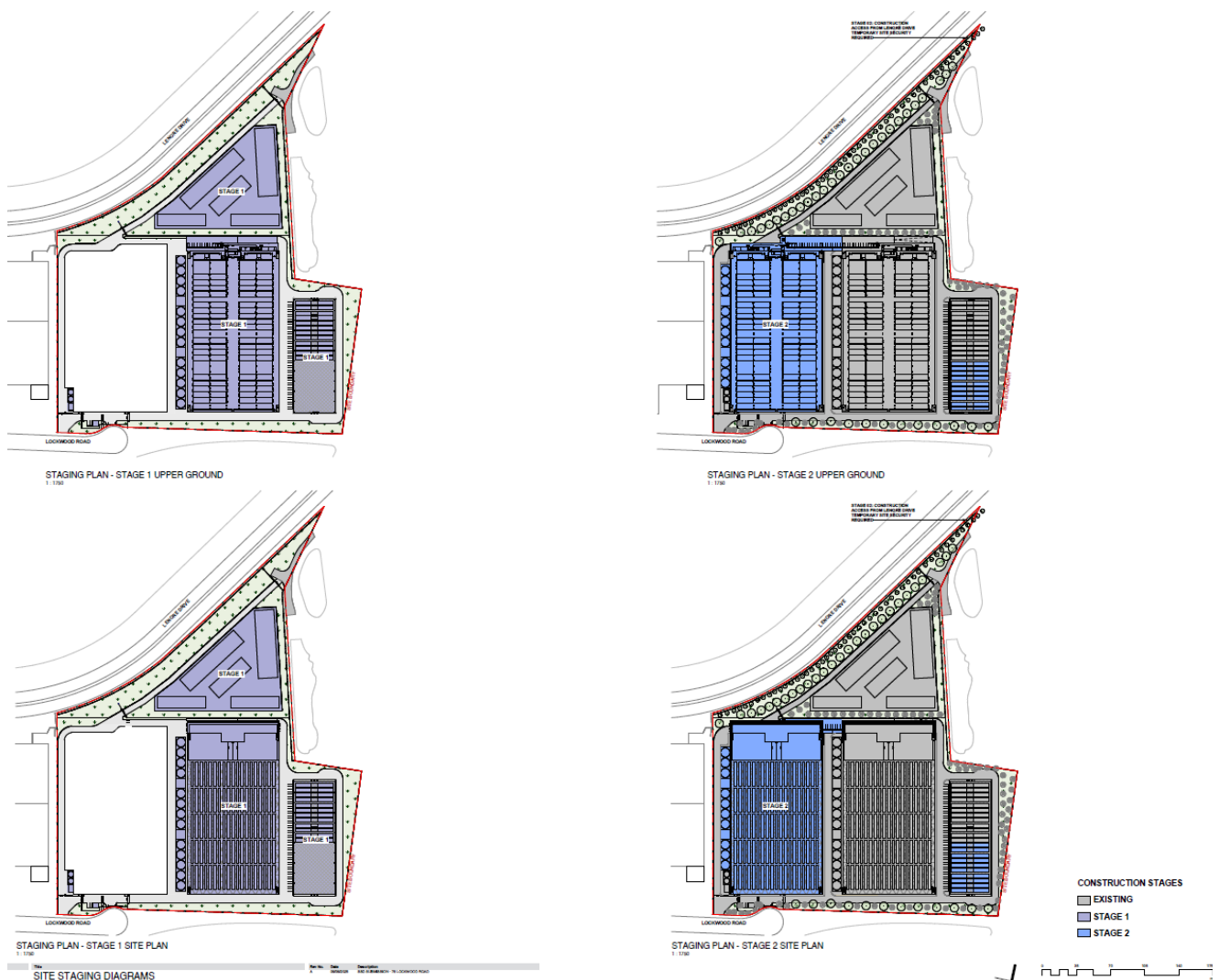
Figure 32 Construction Staging Plans
