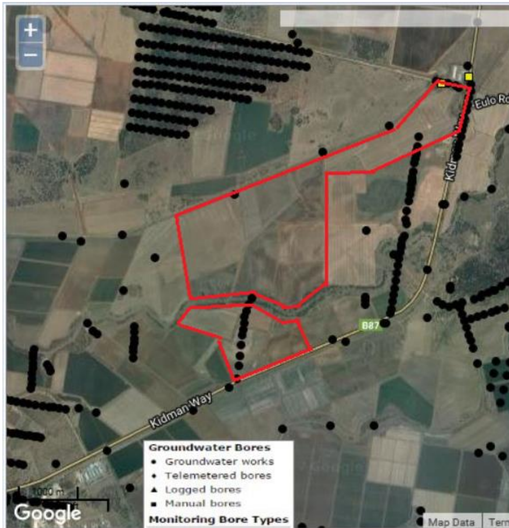
Figure 7-2 Groundwater works in the area (NSW DPI, 2016). The proposal area boundary is indicated by the red line. Monitoring bores are indicated by the yellow boxes.
