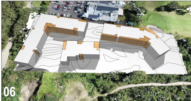
06 Building mass further articulated to provide greater solar access and ventilation to units, whilst reducing building bulk and scale from street and boundaries.
