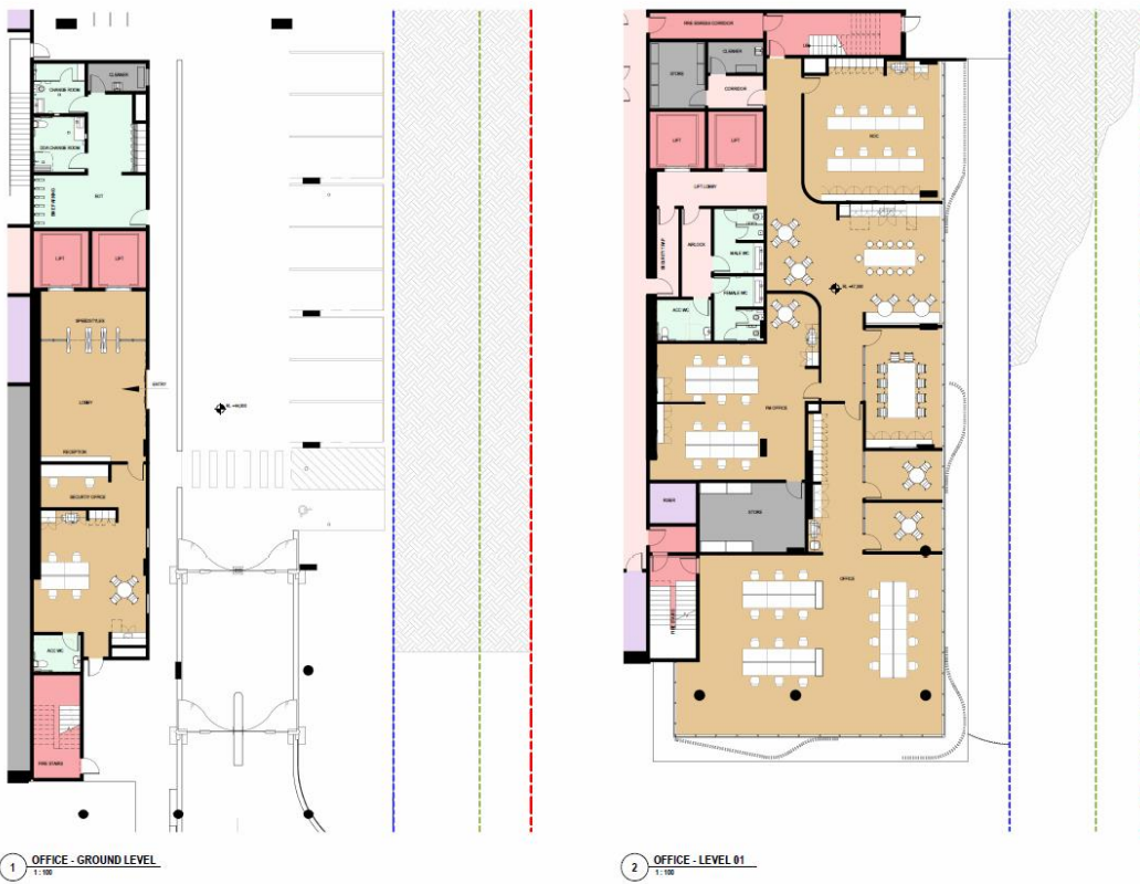
Figure 4 Ground-level and level 1 office floor plans
