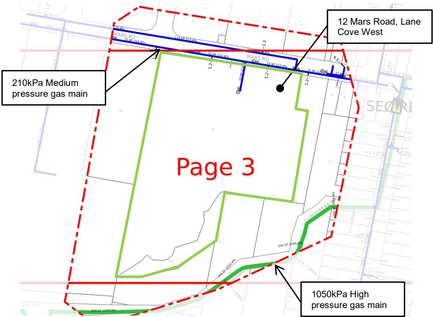
Figure 16 – Existing Jemena Gas Networks Assets around 12 Mars Road, Lane Cove West (Source: BYDA)
