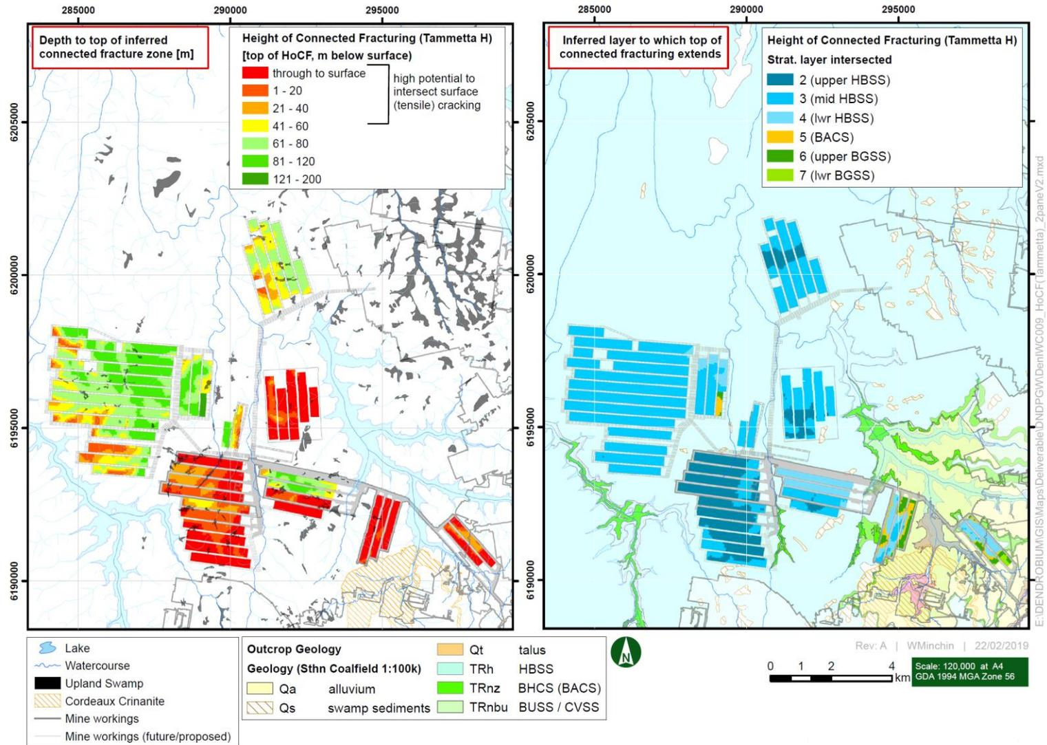
Figure 6-5 Variation in Inferred Height of Fracturing Estimated using the Tammetta Equation [Figure E4 from HydroSimulations, 2019]
