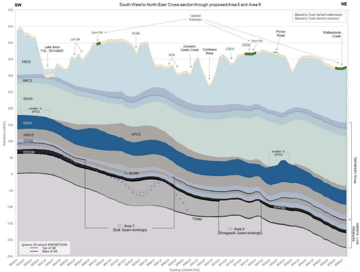
**Plate 6-1 Geological Cross-section through Areas 5 and 6** [Figure 3-4 from HydroSimulations, 2019]
