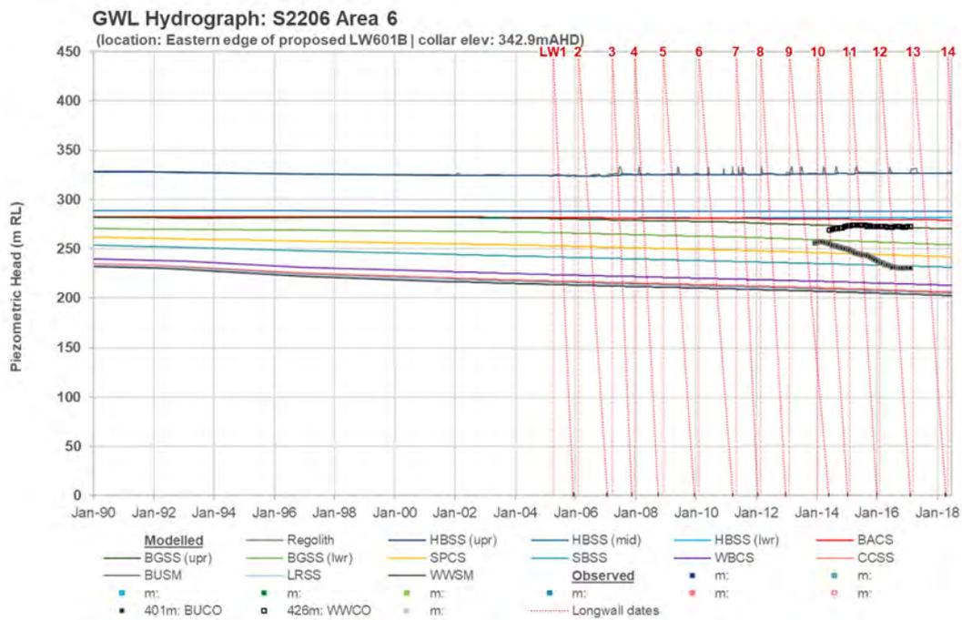
**Figure 7-18 Modelled vs observed groundwater level hydrograph – Bore S2206**
