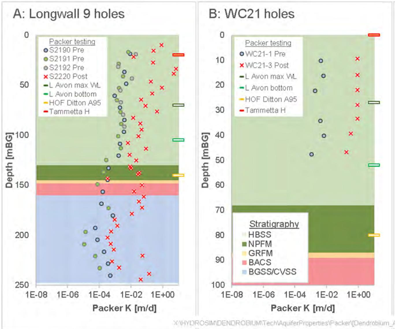
**Figure 4-7 Change in Hydraulic Conductivity (Kh) due to mining – above a longwall**
