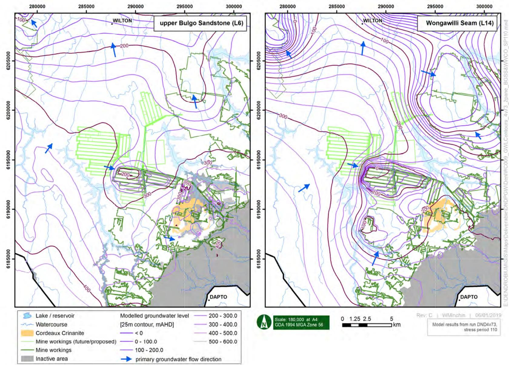
Figure 7-26 Modelled groundwater level contours: model Layers 6 and 14 – mid-2018
