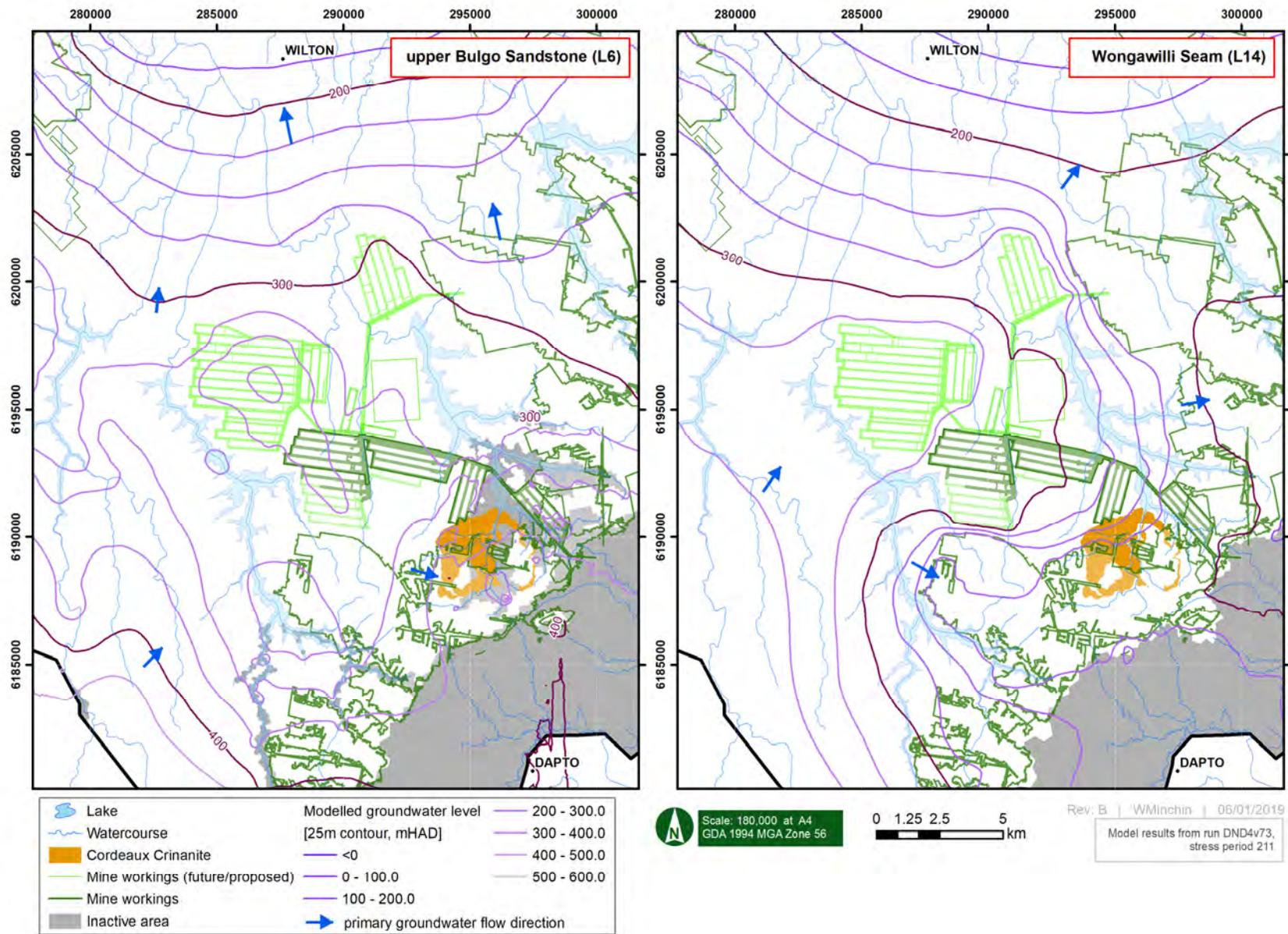
Figure 8-9 Modelled groundwater level contours: model layers 6 and 14 -2200
