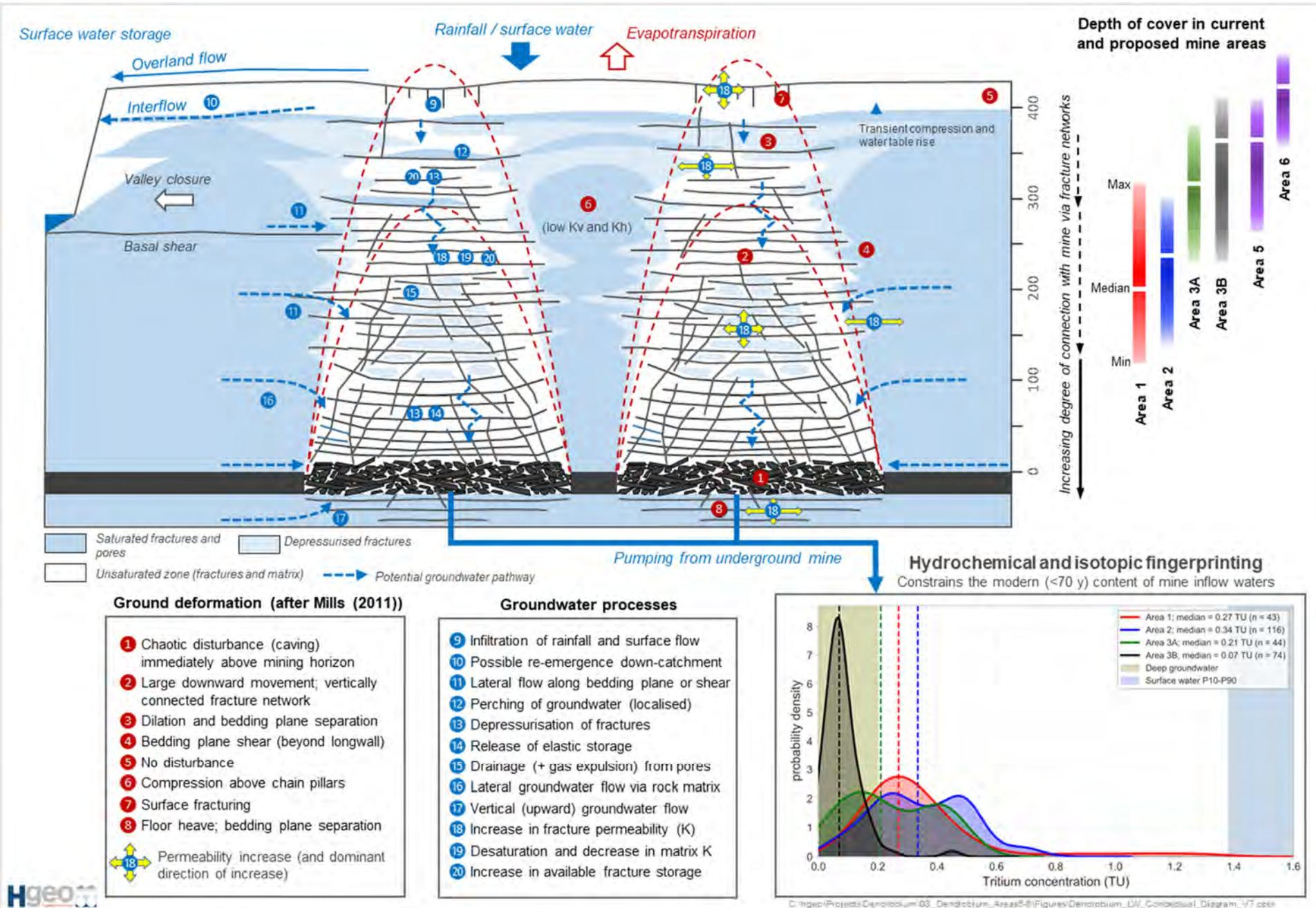
Figure 5-2 Conceptual model: geotechnical and hydrogeological effects of mining at Dendrobium
