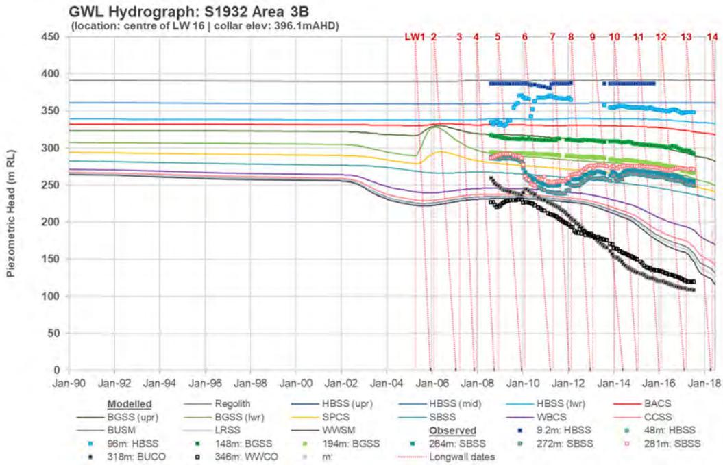
**Figure 7-13 Modelled vs observed groundwater level hydrograph – Bore S1932**
