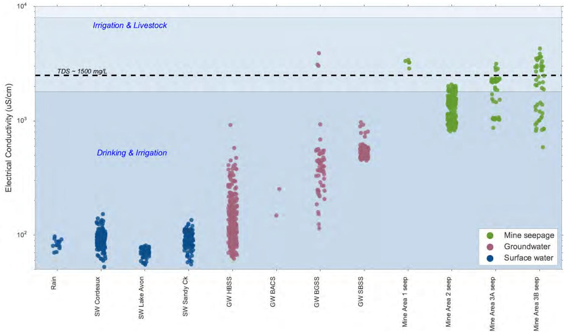
Figure 4-16 Violin plot showing the ranges of EC for various water sources
