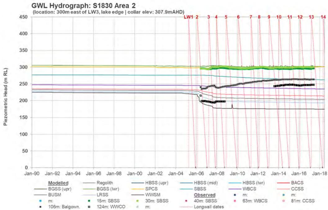
**Figure 7-4 Modelled vs observed groundwater level hydrograph – Bore S1830**
