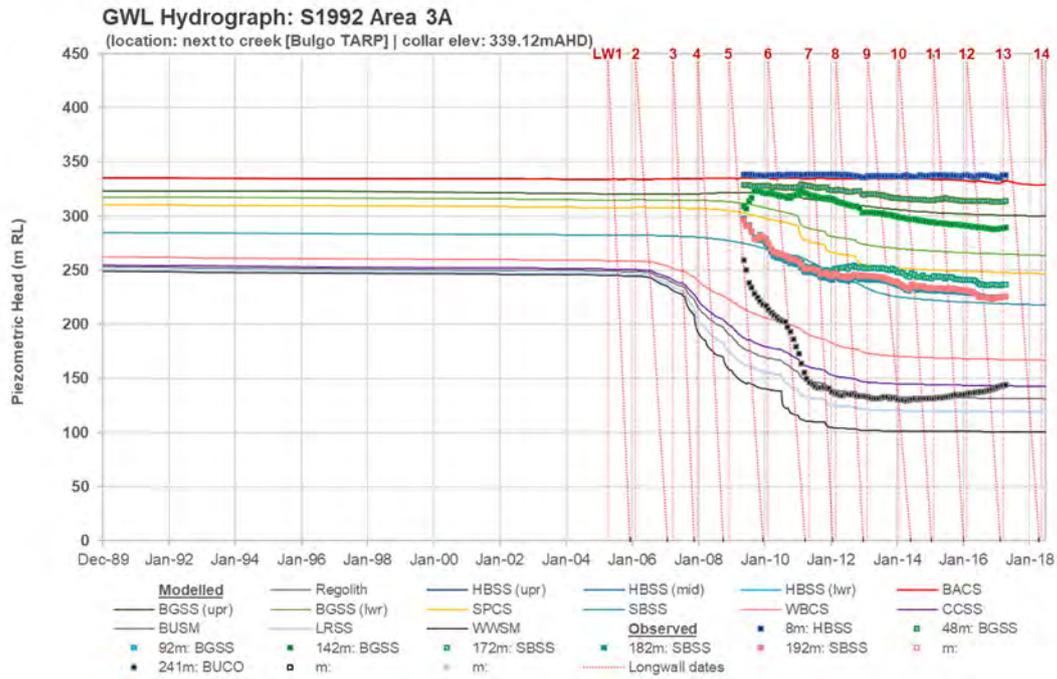
**Figure 7-7 Modelled vs observed groundwater level hydrograph – Bore S1992**
