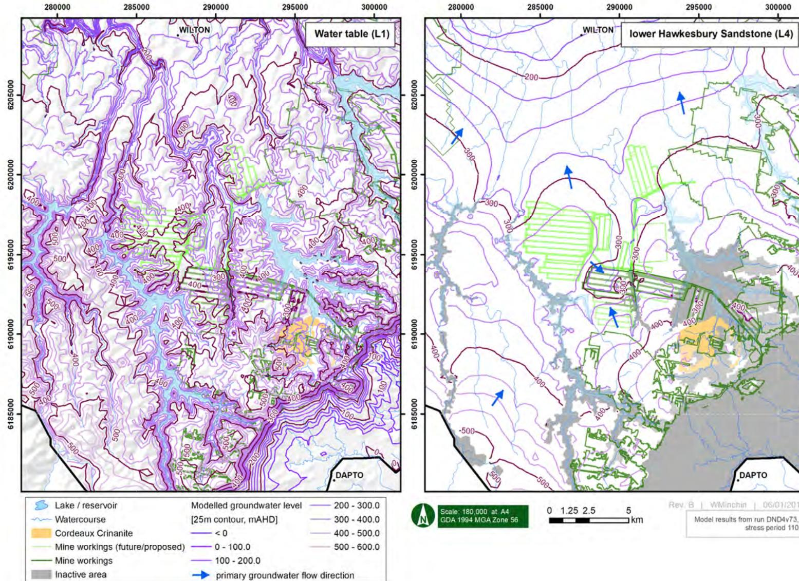
Figure 7-25 Modelled groundwater level contours: model Layers 1 and 4 – mid-2018
