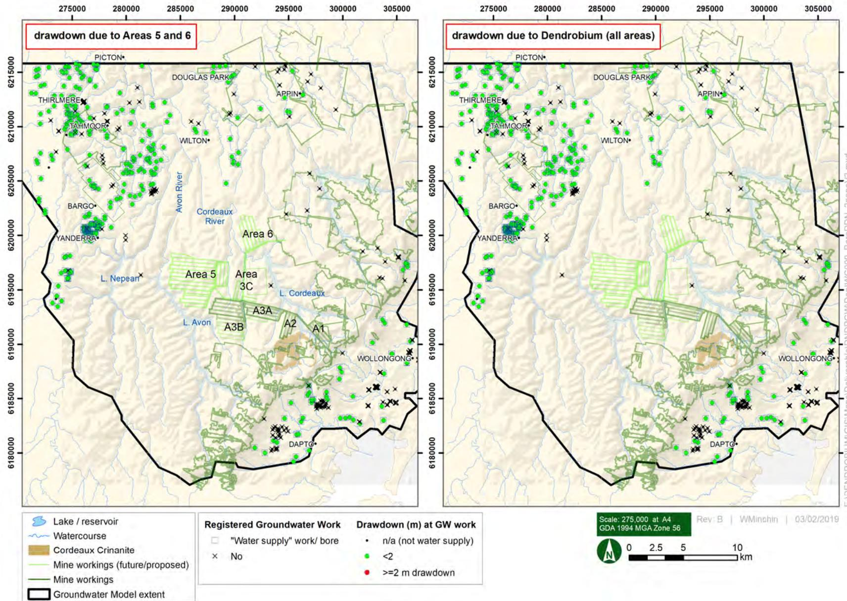
Figure 8-12 Modelled maximum drawdown at Groundwater Works (bores): Dendrobium
