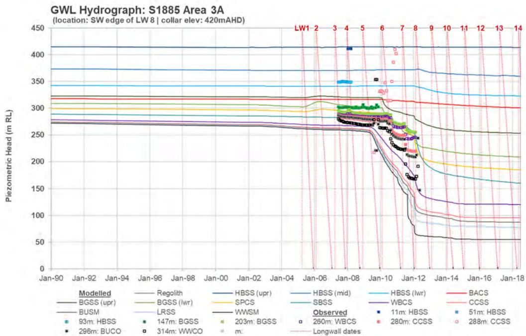
**Figure 7-8 Modelled vs observed groundwater level hydrograph – Bore S1885**
