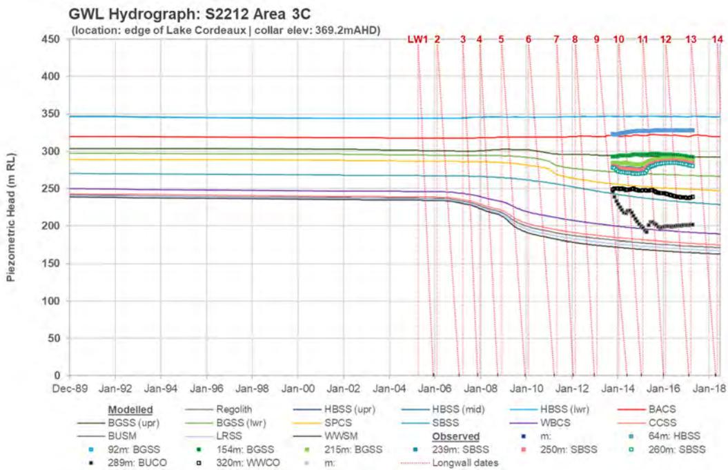
**Figure 7-16 Modelled vs observed groundwater level hydrograph – Bore S2212**
