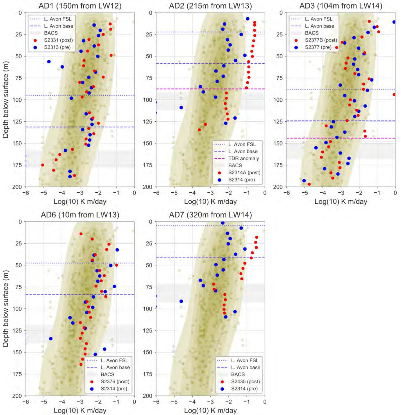
**Figure 4-8 Change in hydraulic conductivity (Kh) due to mining – off-goaf areas**
