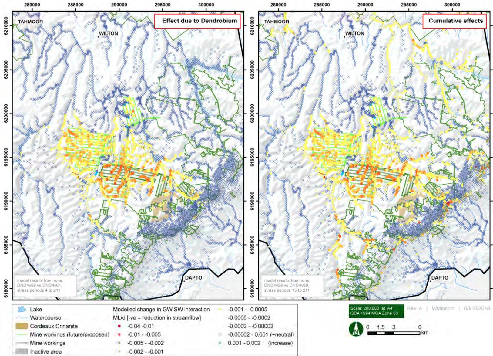
**Figure 8-14 Predicted distribution of stream flow depletion**
