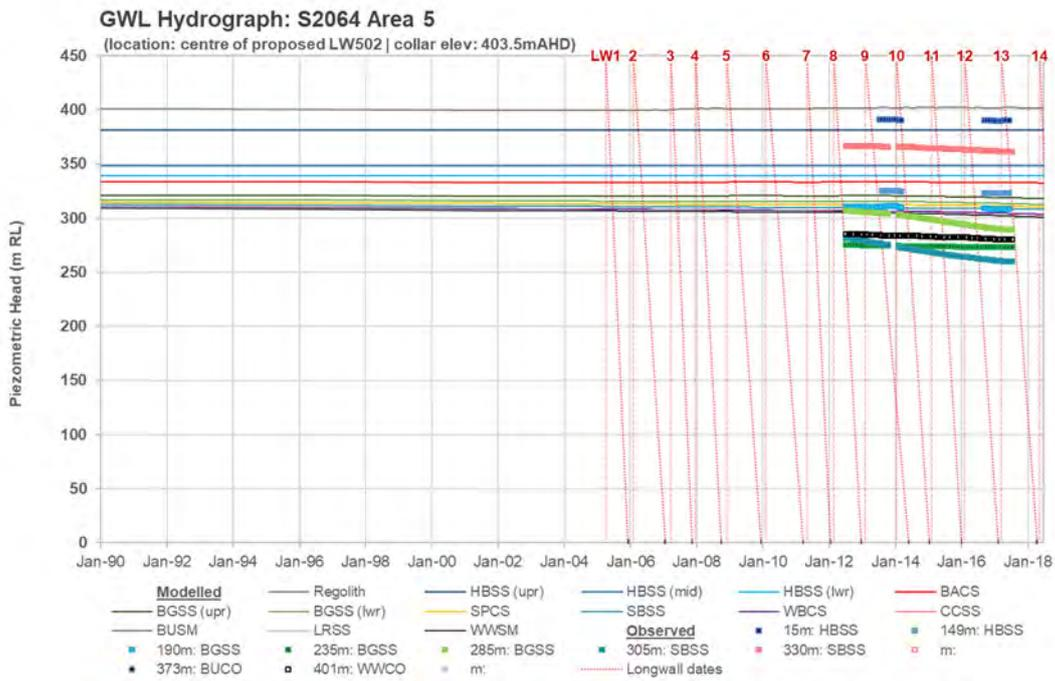
**Figure 7-15 Modelled vs observed groundwater level hydrograph – Bore S2064**
