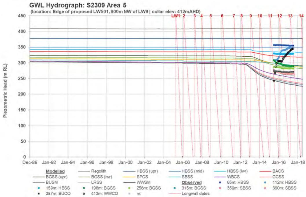
**Figure 7-19 Modelled vs observed groundwater level hydrograph – Bore S2309**
