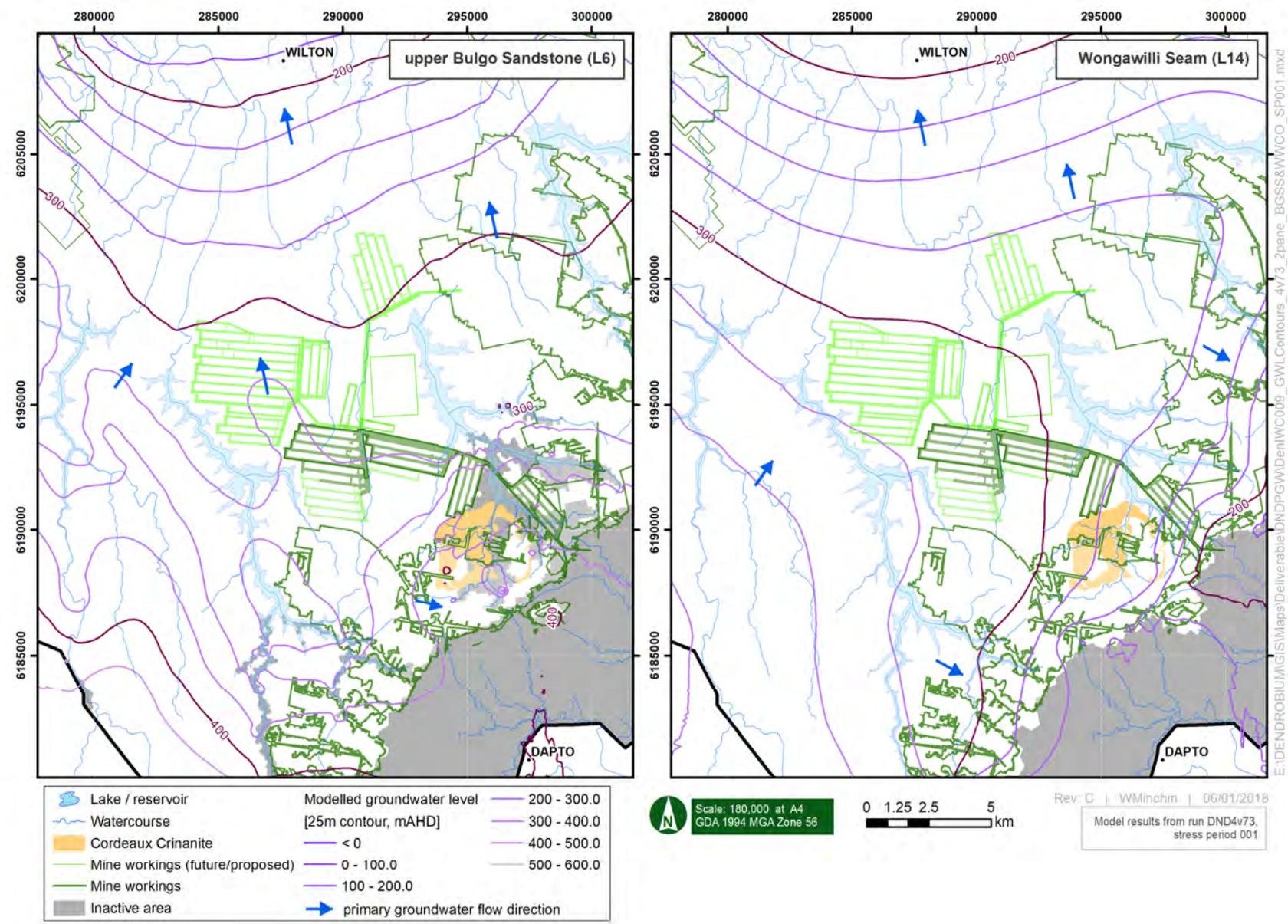
**Figure 7-24** Modelled groundwater level contours: model Layers 6 and 14 – pre-mining
