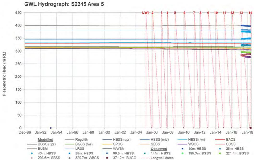
**Figure 7-20 Modelled vs observed groundwater level hydrograph – Bore S2345**
