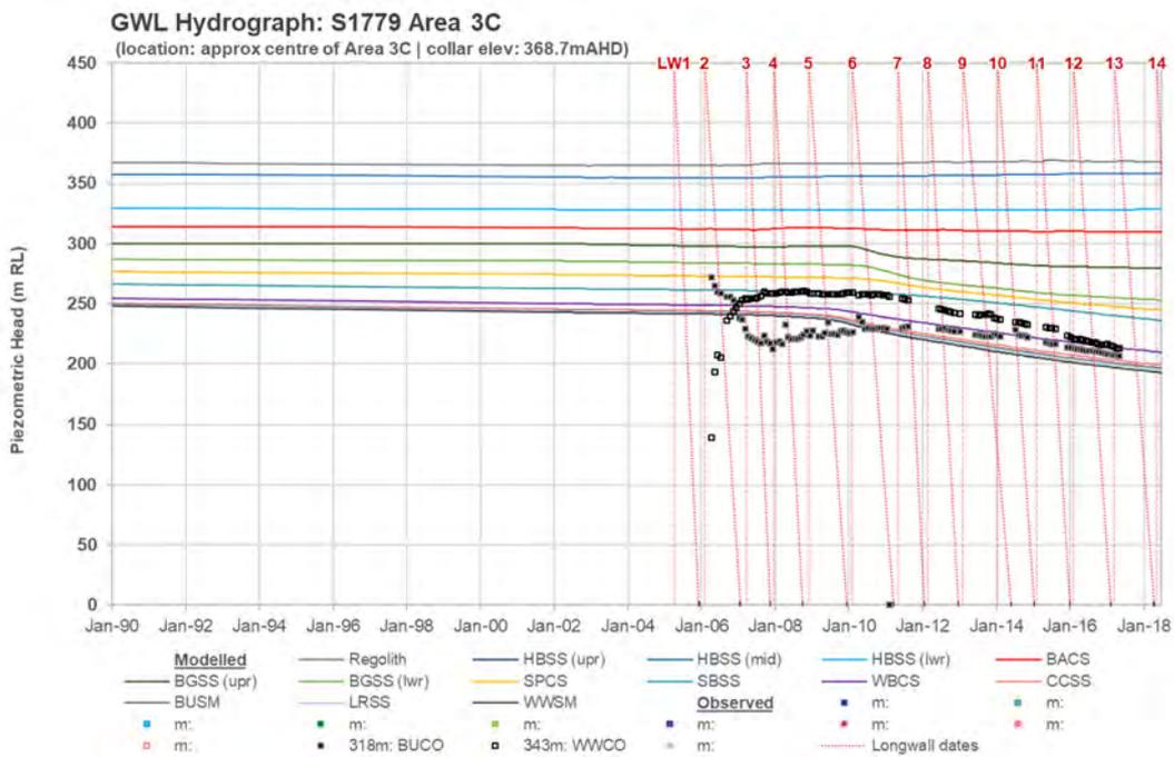
**Figure 7-14 Modelled vs observed groundwater level hydrograph – Bore S1779**
