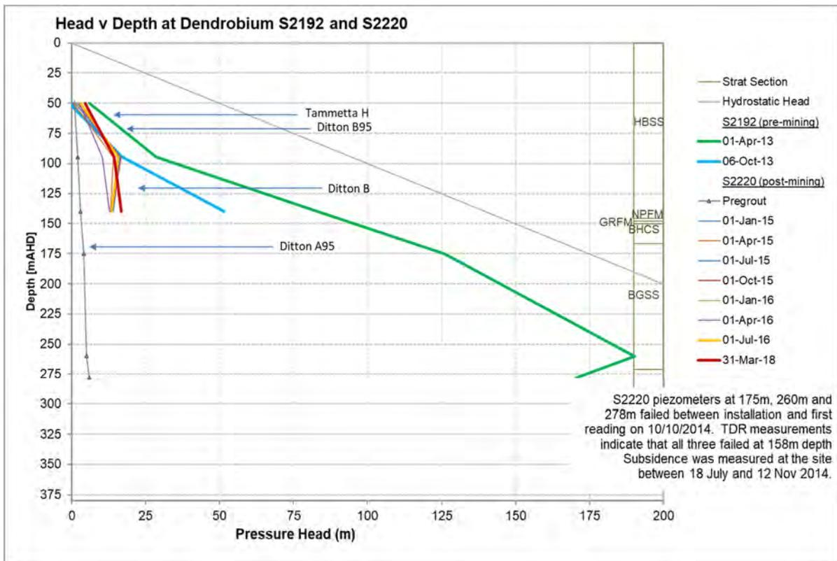
Figure 4-13 Groundwater Levels above Longwall 9: A] Pressure Head; B] Head vs Depth
