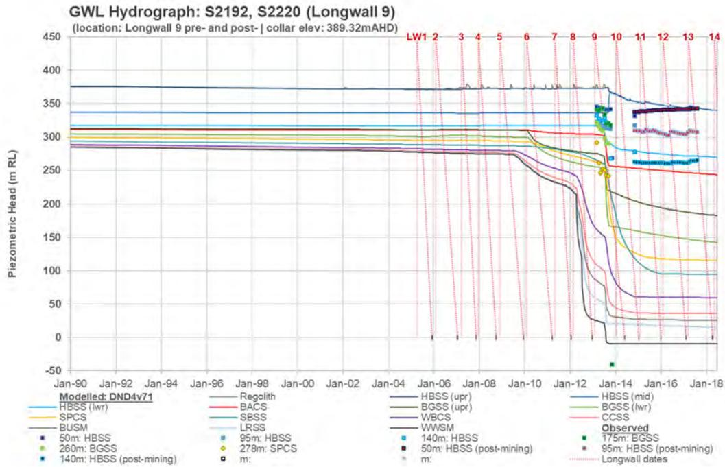
**Figure 7-9 Modelled vs observed groundwater level hydrograph – Bore S2192-S2220 (LW9)**
