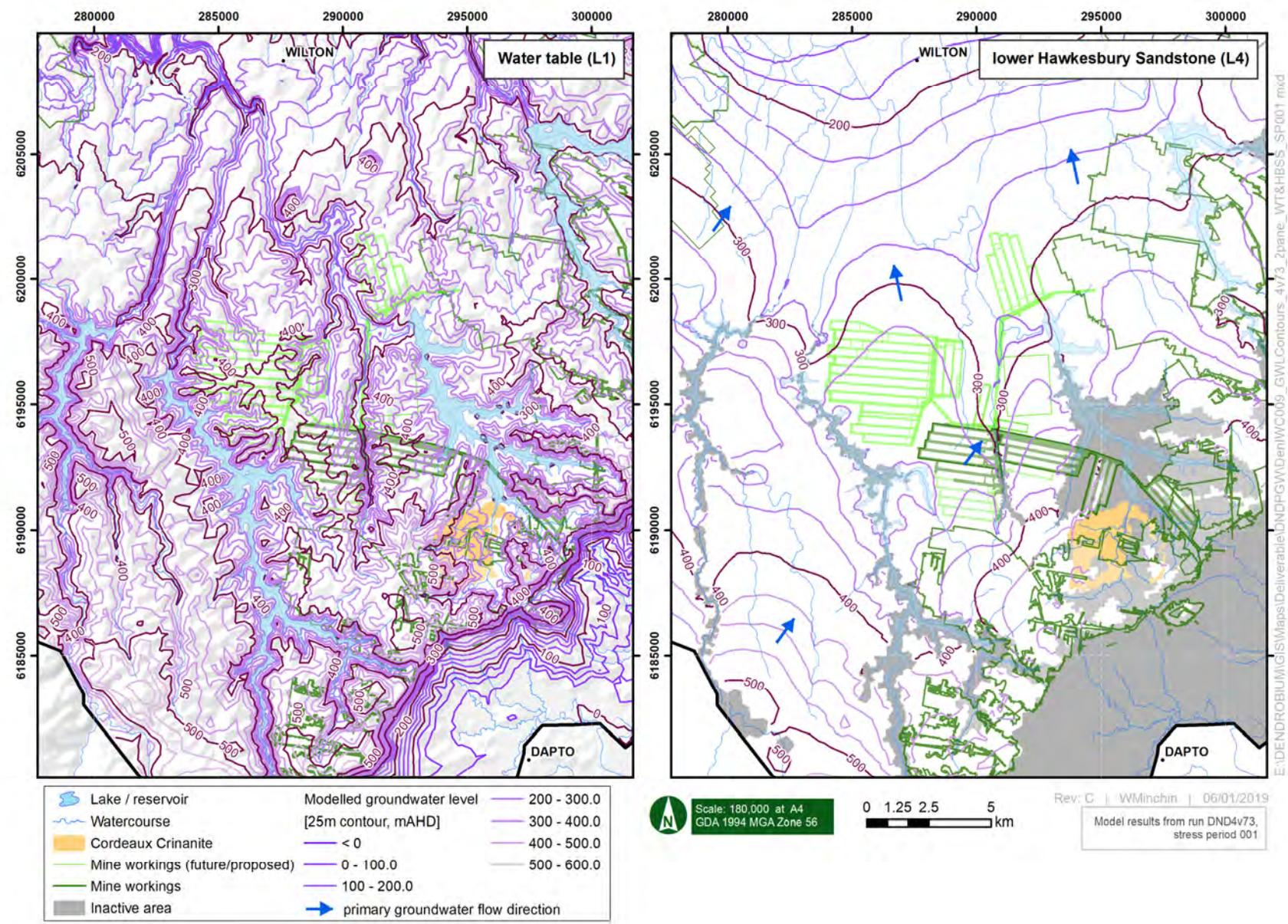
Figure 7-23 Modelled groundwater level contours: model Layers 1 and 4 – pre-mining
