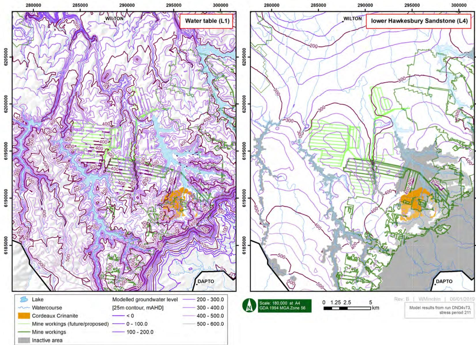
Figure 8-8 Modelled groundwater level contours: model layers 1 and 4 -2200
