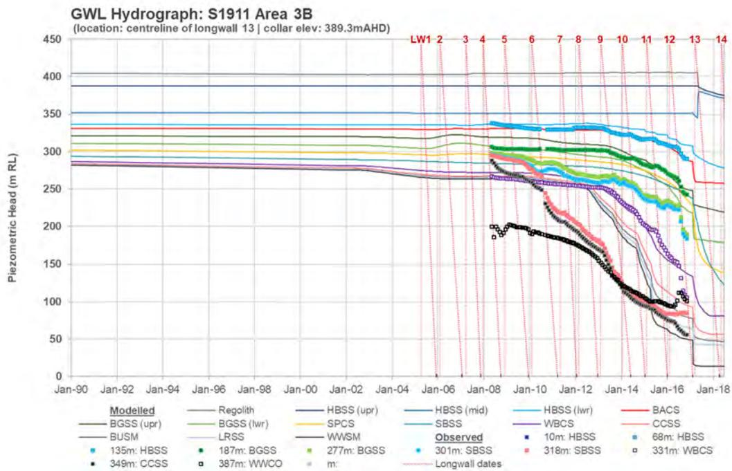
**Figure 7-10 Modelled vs observed groundwater level hydrograph – Bore S1911**
