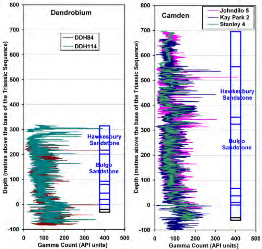
Figure 10. Downhole gamma logs for the bores in the Dendrobium and Camden areas.
