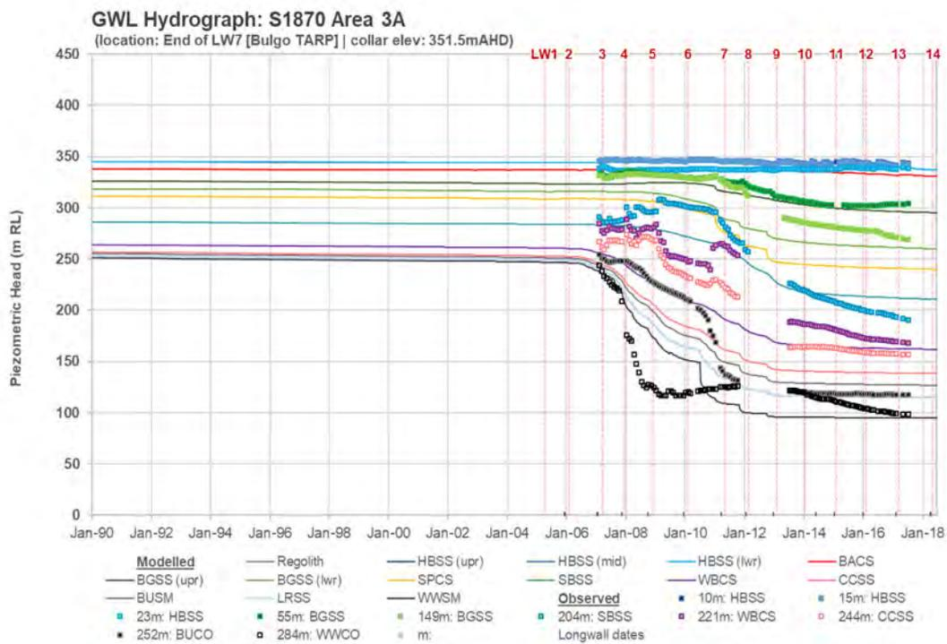
**Figure 7-6 Modelled vs observed groundwater level hydrograph – Bore S1870**
