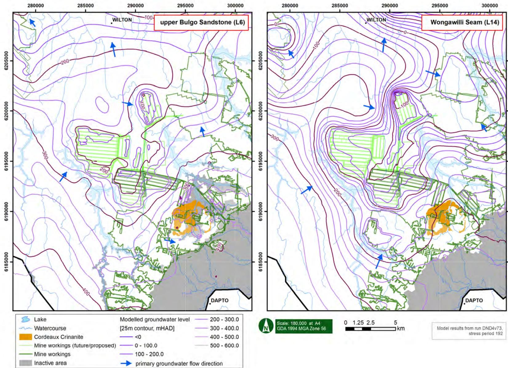
**Figure 8-7 Modelled groundwater level contours: model layers 6 and 14 -2049**
