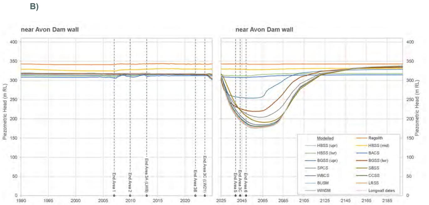
**Figure 8-4 Predicted groundwater levels – hydrographs in and near Area 5**
