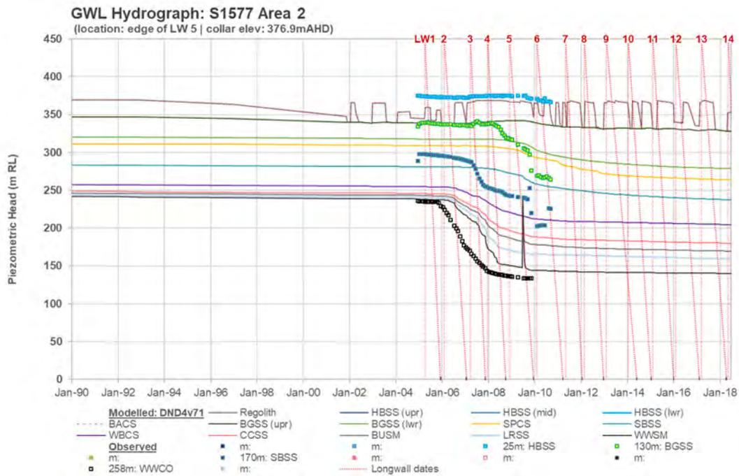
**Figure 7-5 Modelled vs observed groundwater level hydrograph – Bore S1577**
