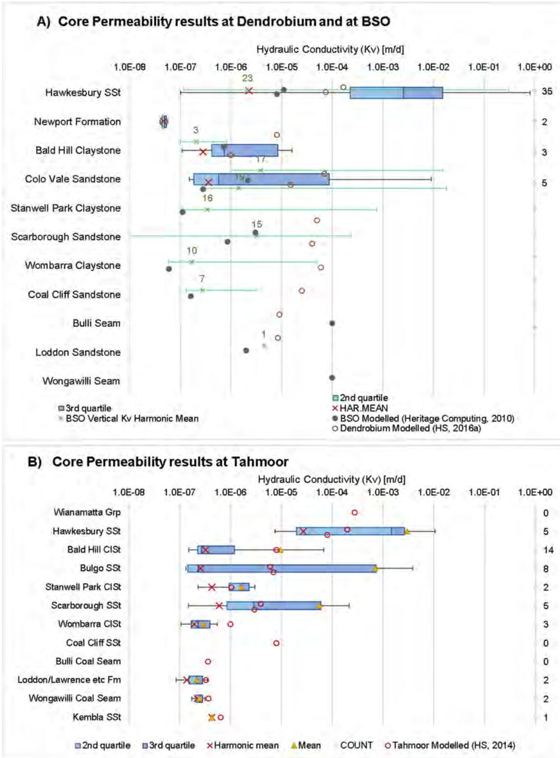
Figure 4-4 Hydraulic conductivity (Kv) from core testing
