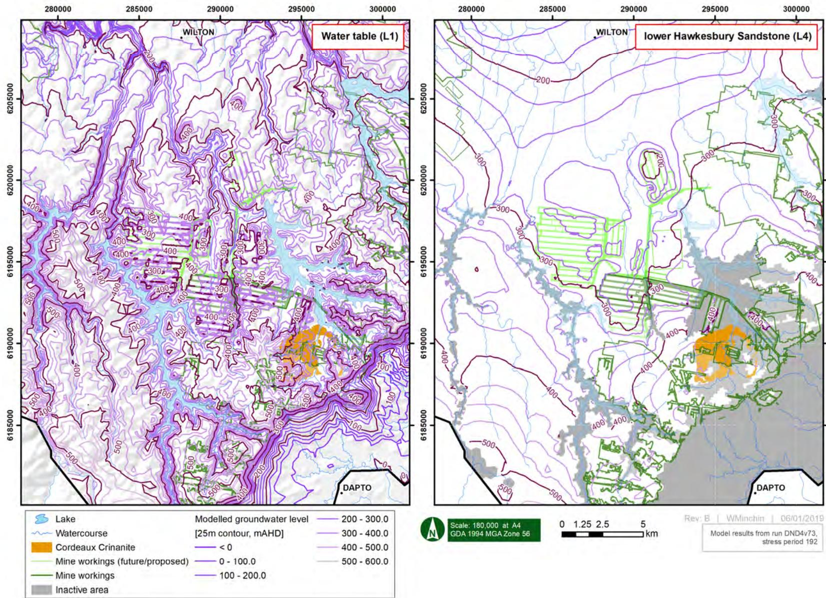
Figure 8-6 Modelled groundwater level contours: model Layers 1 and 4 – 2049
