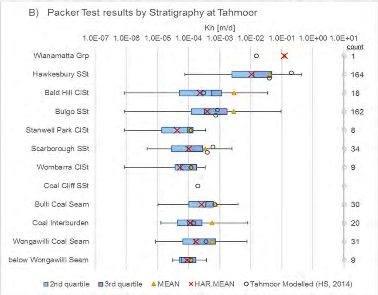
Figure 4-3 Summary of Horizontal Hydraulic Conductivity (Kh) by Stratigraphic unit
