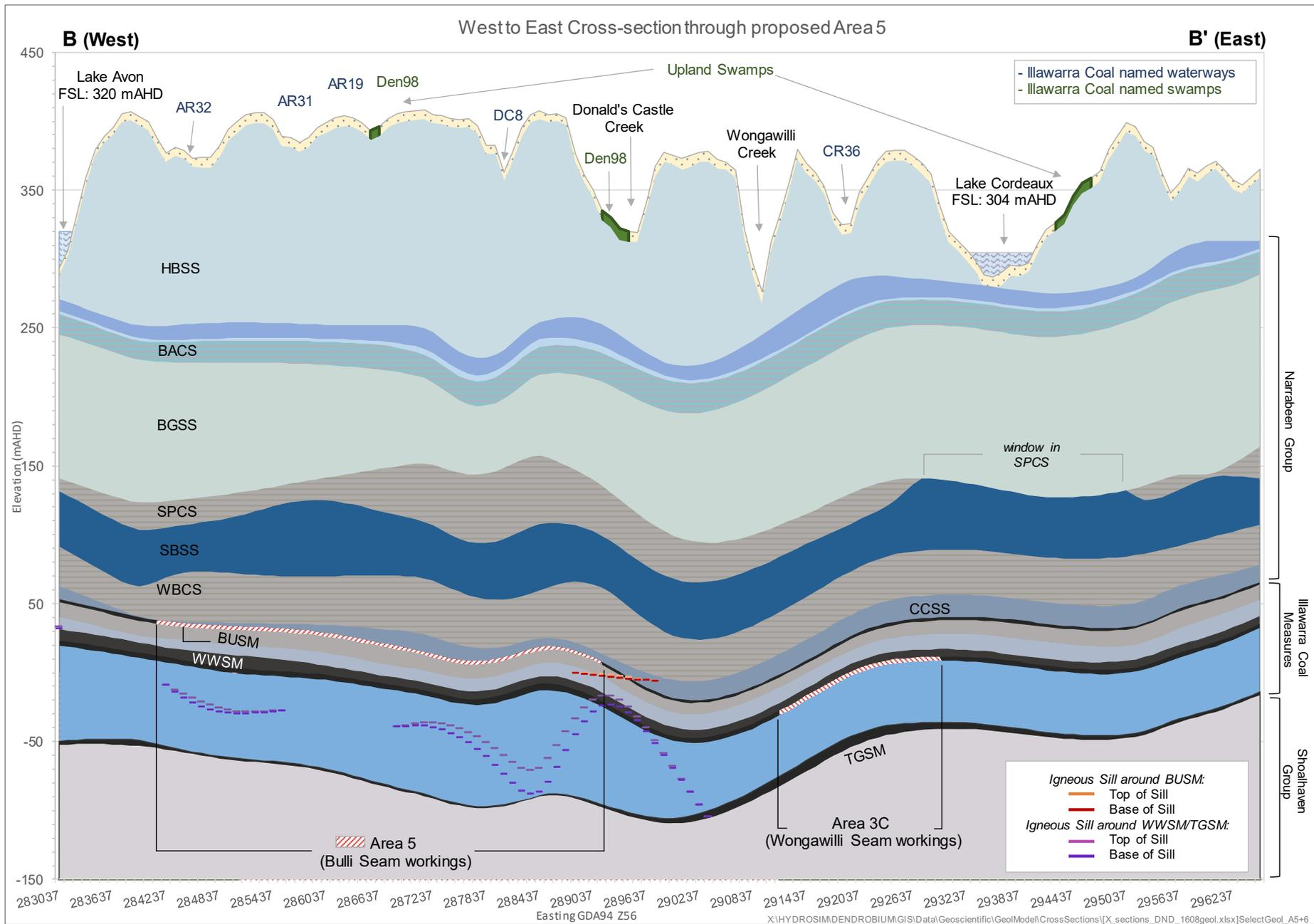
**Figure 3-5 Geological Cross-section: West-East through Area 5**
