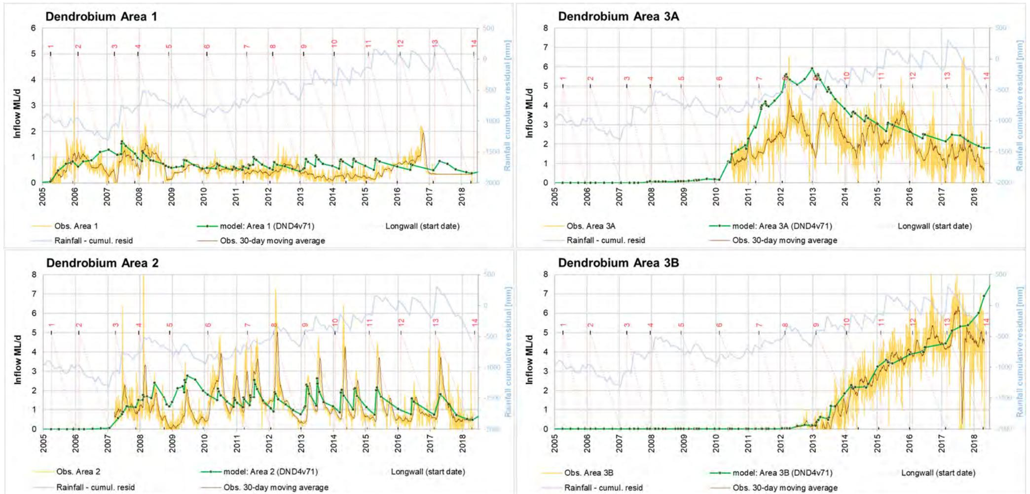
**Figure 7-27 Modelled vs observed Mine Inflow by Area**
