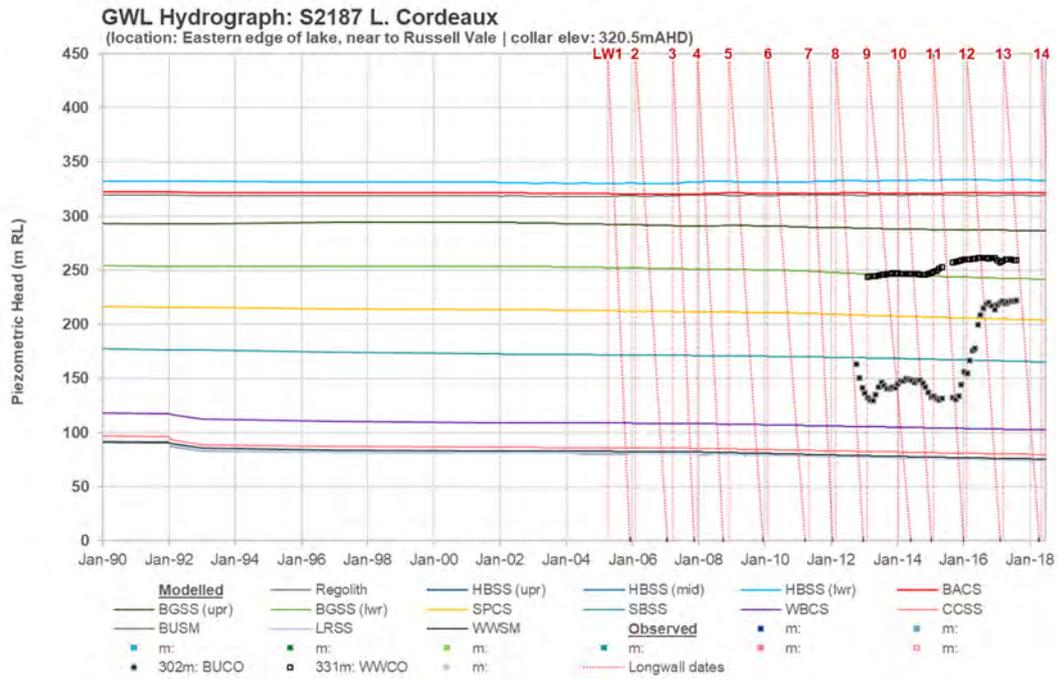
**Figure 7-17 Modelled vs observed groundwater level hydrograph – Bore S2187**
