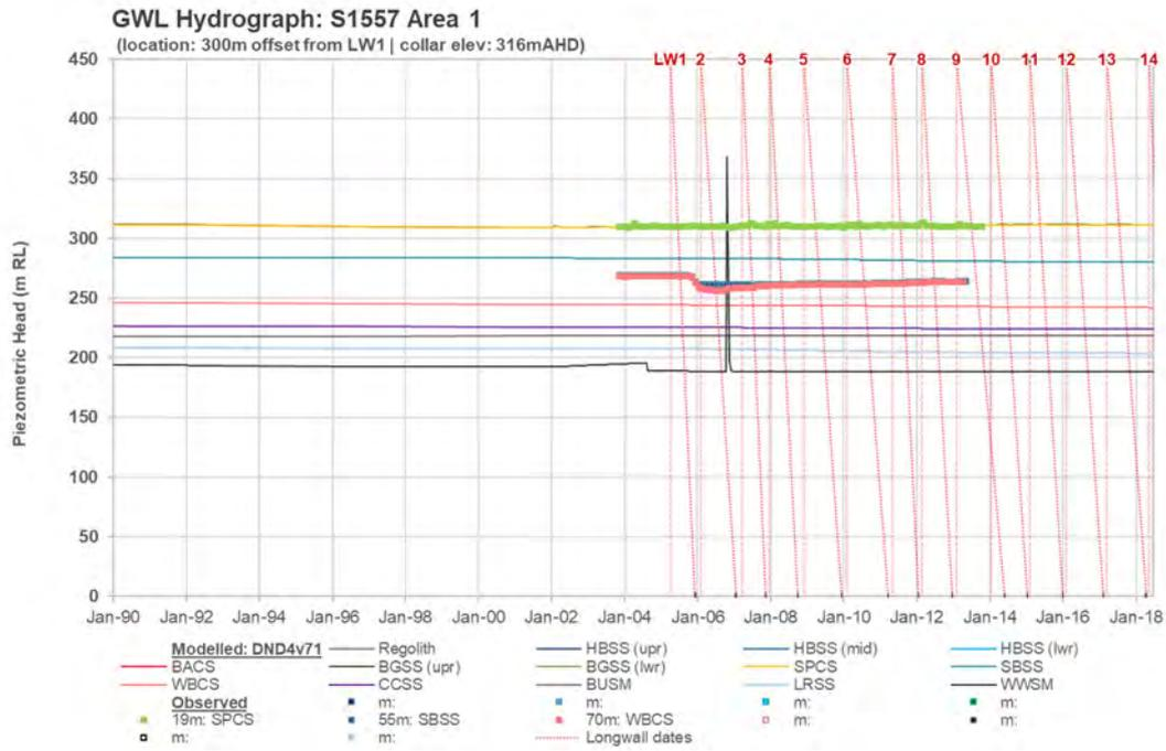
**Figure 7-3 Modelled vs observed groundwater level hydrograph – Bore S1557**
