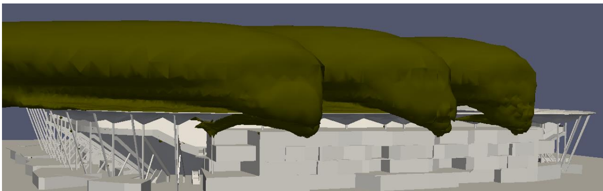
Figure 7: Kitchen exhaust plume at 1:300 dilution viewed from West-North-West
