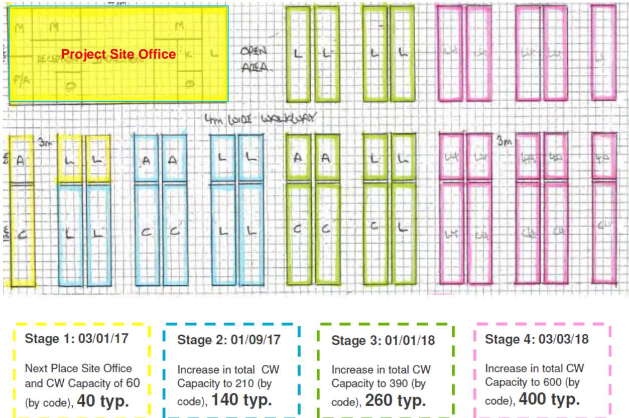
Figure 6 – Site Construction Amenities
