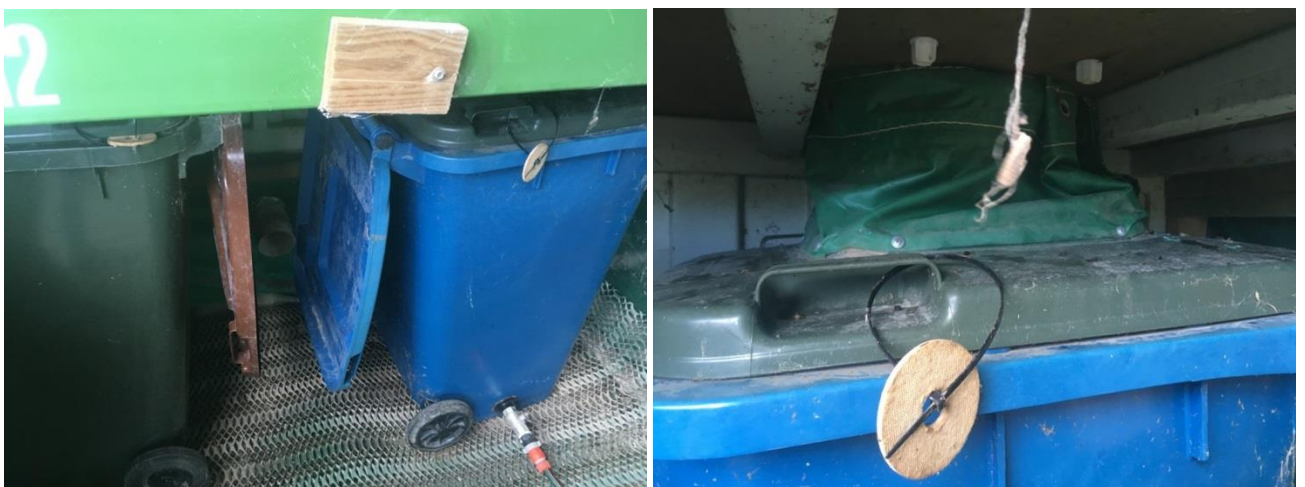
Photograph 2: Wheelie bins in action. Seepage pipe at the base, with flexible collar to separate lid while in operation.
