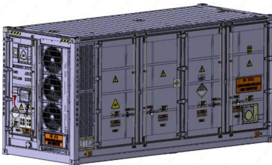
Figure 3.2 Example battery container unit
