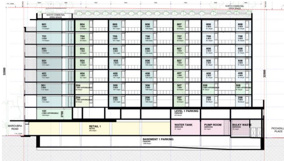
FIGURE 7: SECTION DEPICTING GROUND FLOOR USES, PARKING ARRANGEMENT AND INTERFACE AT THE STREET.
