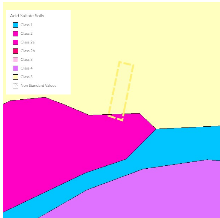
Figure 1: Screenshot from www.planningportal.nsw.gov.au showing Class 5 & 2 ASS at the site location.
