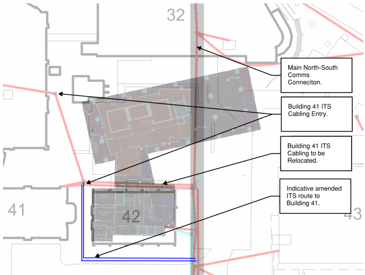
Figure 7: Proposed ITS Services Diversions Diagram
