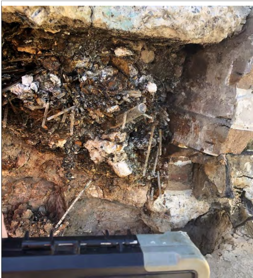
Photo 7: Glass tubes represent possible capacitors within fill materials on Stage 2 (source anticipated to be former electrical manufacturing business). Anecdotal evidence indicates PCBs at around 180mg/kg in this area.
