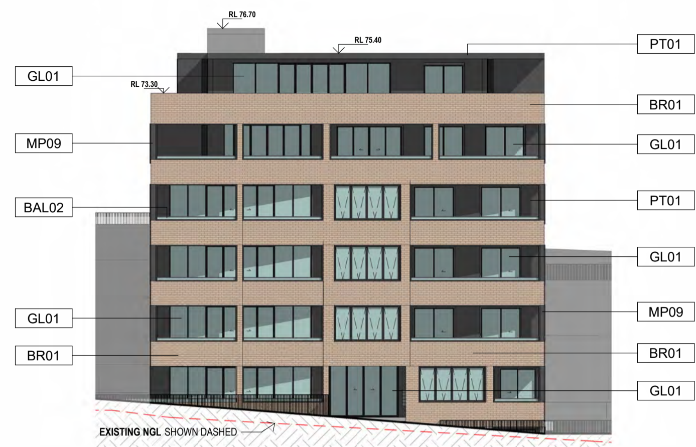
1 BLD N - NORTH ELEVATION 1 : 200
