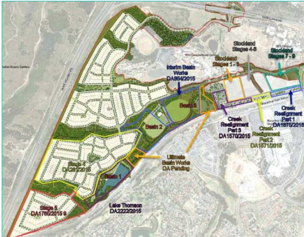
Figure 4 - Regional Stormwater Management (JWP, Nov 2017)
