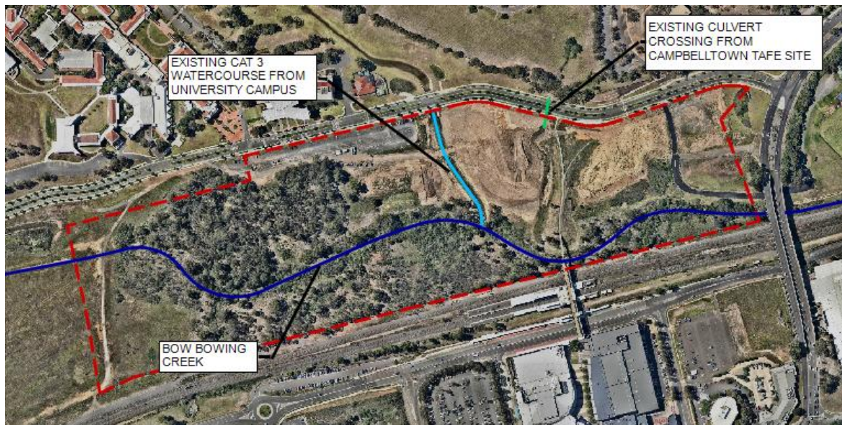
Figure 3 - Existing Drainage Layout
