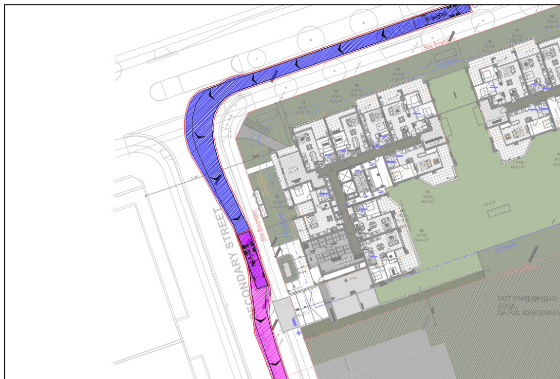
Figure 4 Swept path analysis – on-street loading zone
