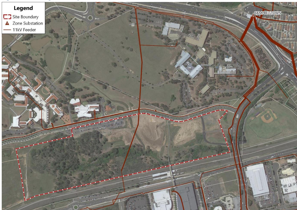
Figure 8 - Existing Electricity Network
