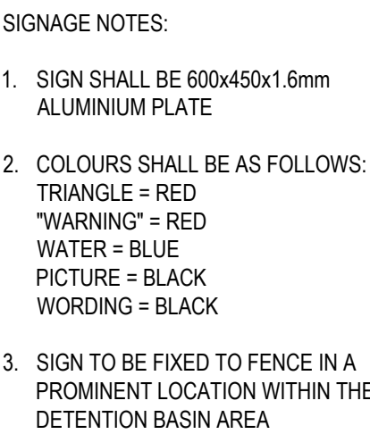
ON SITE STORMWATER DETENTION WARNING SIGN
