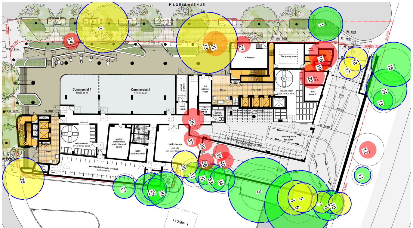
Figure 47 Tree Removal and Retention Plan
