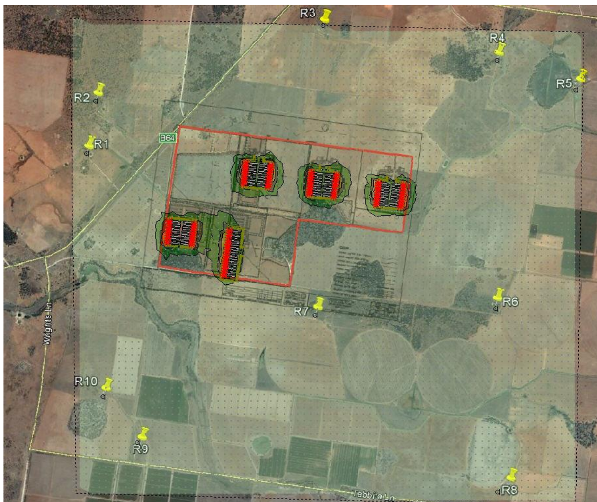
Figure II-4: Predicted E/N period L_{Aeq, 15\text{minute}} noise levels - Operation of Fans. Neutral Conditions
