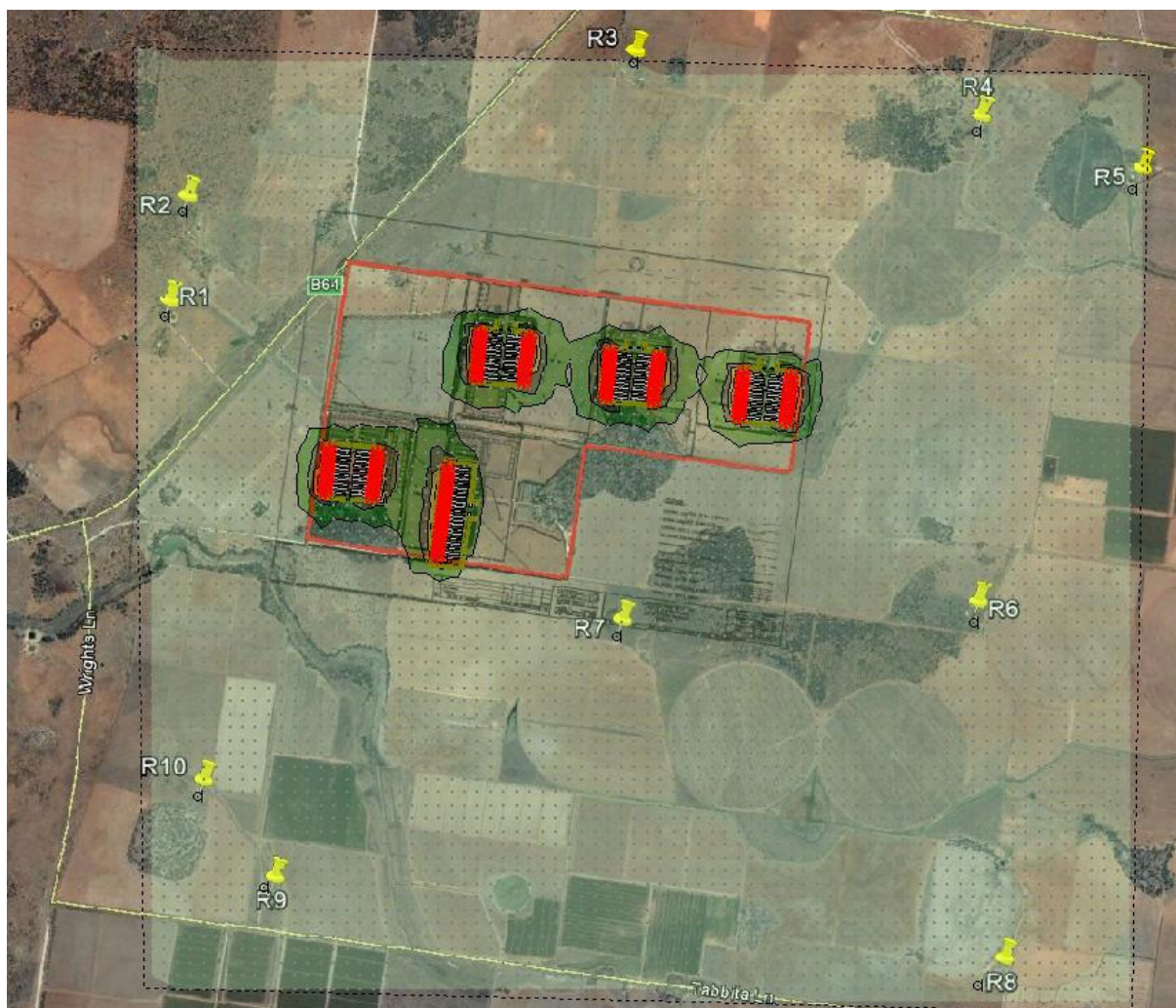
Figure II-3: Predicted Day period L_{Aeq, 15\text{minute}} noise levels - Operation of Fans. Neutral Conditions
