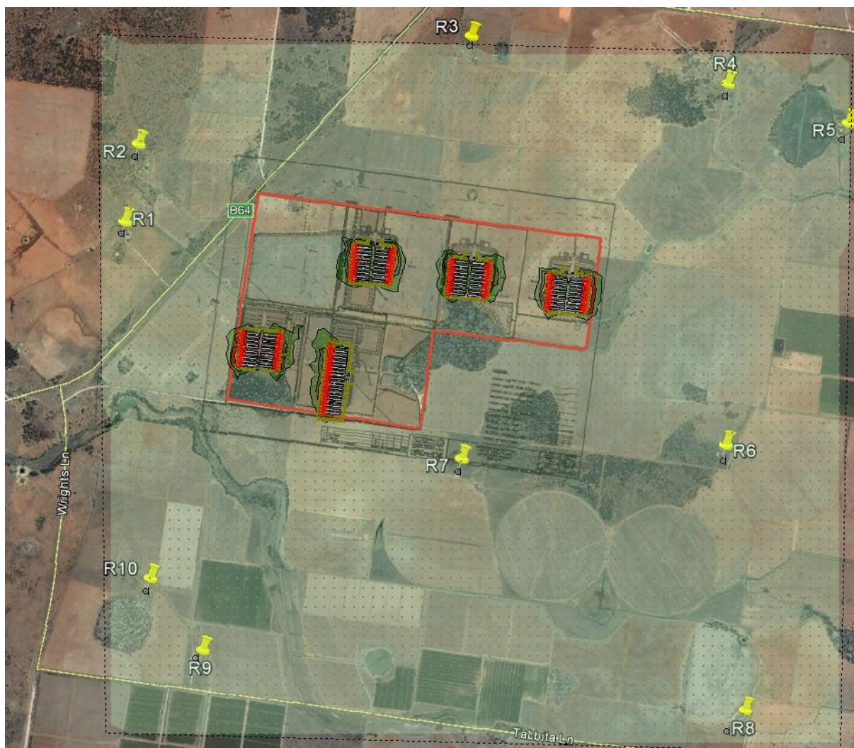
Figure II-5: Predicted E/N period L_{Aeq, 15\text{minute}} noise levels - Operation of Fans. Adverse Conditions
