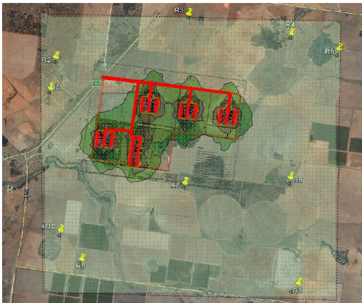
Figure II-7: Predicted night period L_{Aeq, 15\text{minute}} noise level - Feed Delivery and Silo Refilling. Adverse Conditions
