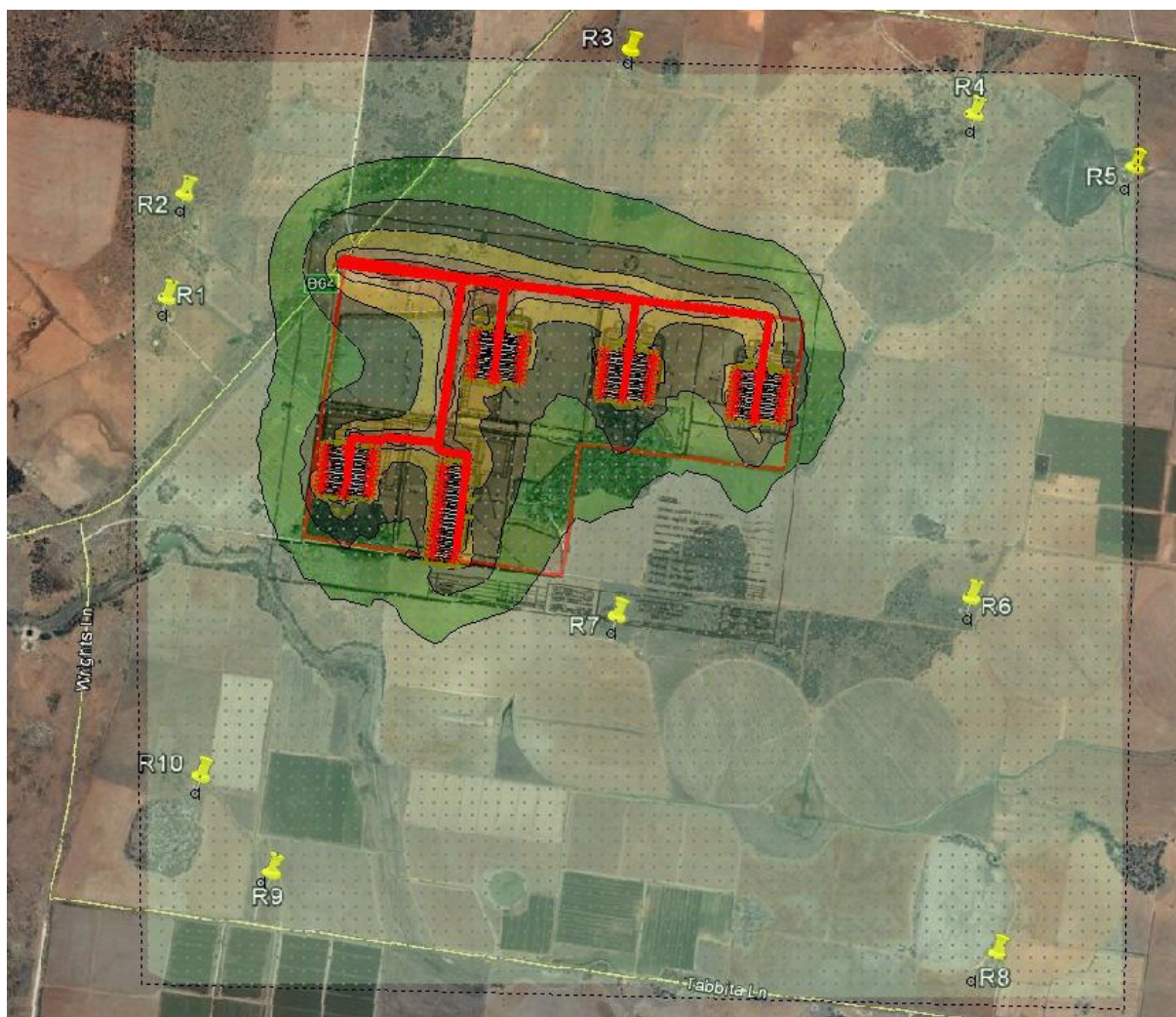
Figure II-8: Predicted night period L_{Aeq, 15\text{minute}} noise levels - Bird Collection, Adverse Conditions
