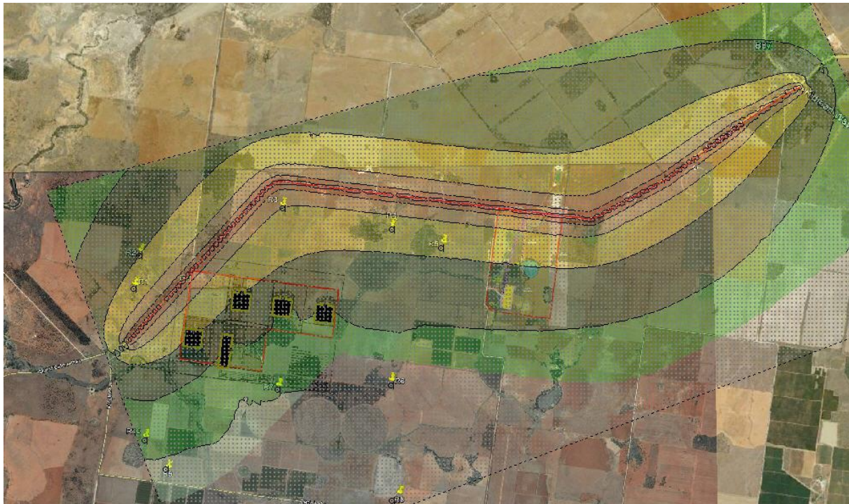
Figure II-10: Predicted L_{Aeq, period} noise levels - Additional Traffic Movements
