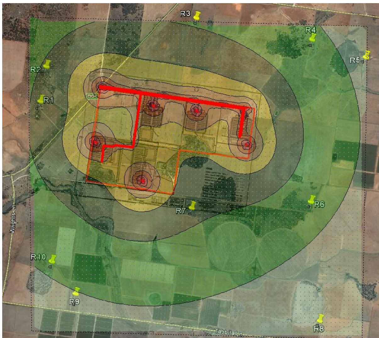
Figure II-1: Predicted Day period L_{Aeq, 15\text{minute}} noise levels - Bulk Earthworks
