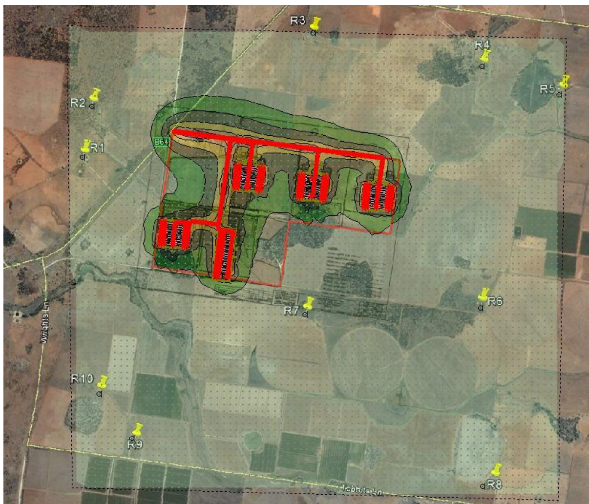
Figure II-6: Predicted day period L_{Aeq, 15\text{minute}} noise level - Feed Delivery and Silo Refilling. Neutral Conditions
