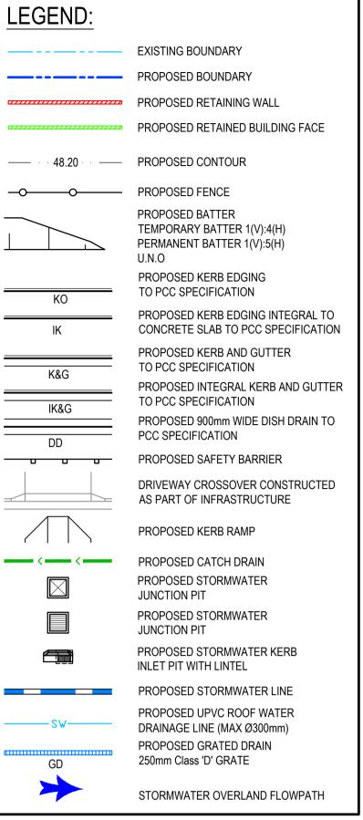
ALL LEVELS SHOWN ARE ± 1000mm ROOF WATER DOWN PIPE LOCATIONS TO BE CONFIRMED
