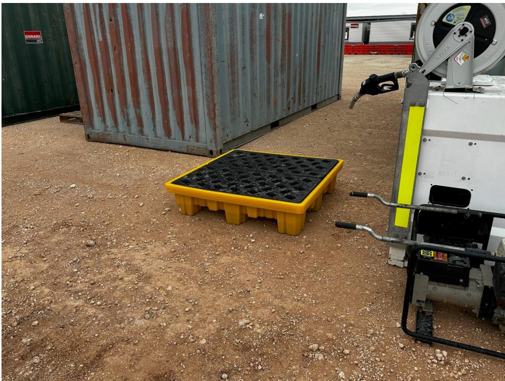
Photo 6: Mobile Spill control bund
