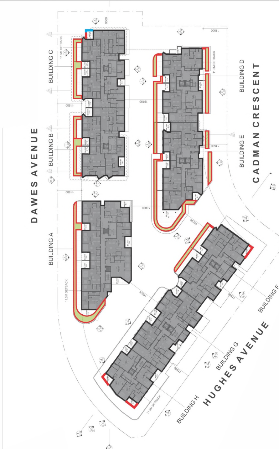
Figure 5: Recommended Treatment for the Level 4 Terraces
