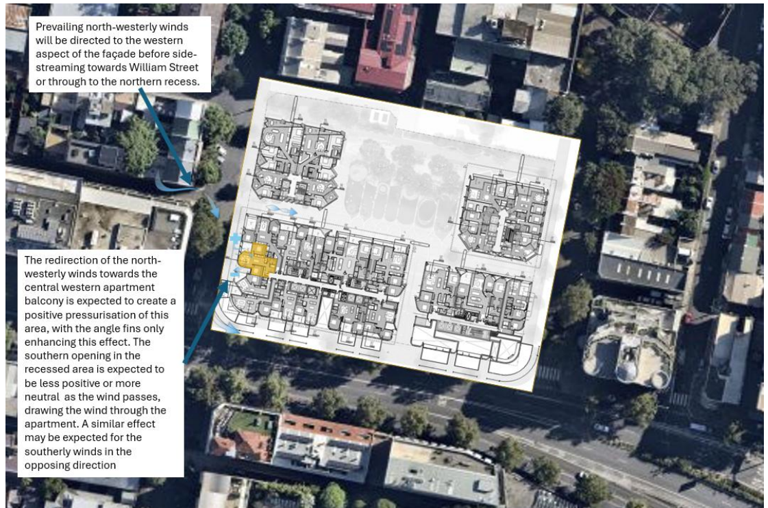
Figure 4: Expected Wind Flow During North-Westerly and Southerly Winds for Natural Ventilation
