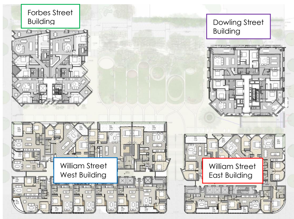
FIGURE 1-4 – TYPICAL FLOOR LEVEL (LEVEL 01-02)
