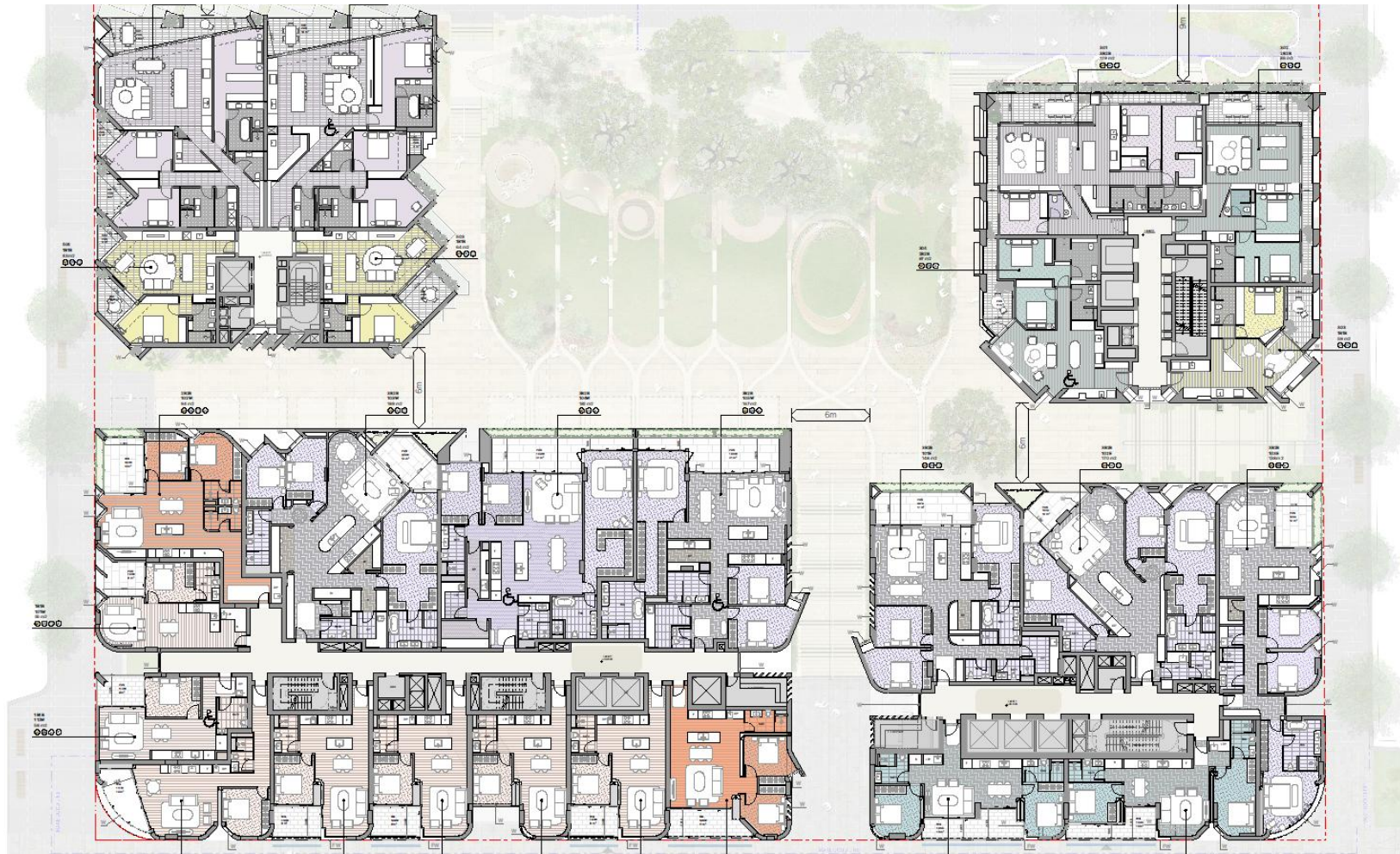
Solar Access through sensible plan layout and form (typical level) - 164-194 William St, Woolloomooloo 2011
