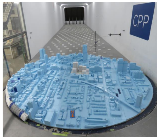
Figure 3a: Photographs of Wind Tunnel Test and Surrounds Model looking south – Configurations A (top), B (middle), and C (bottom)
