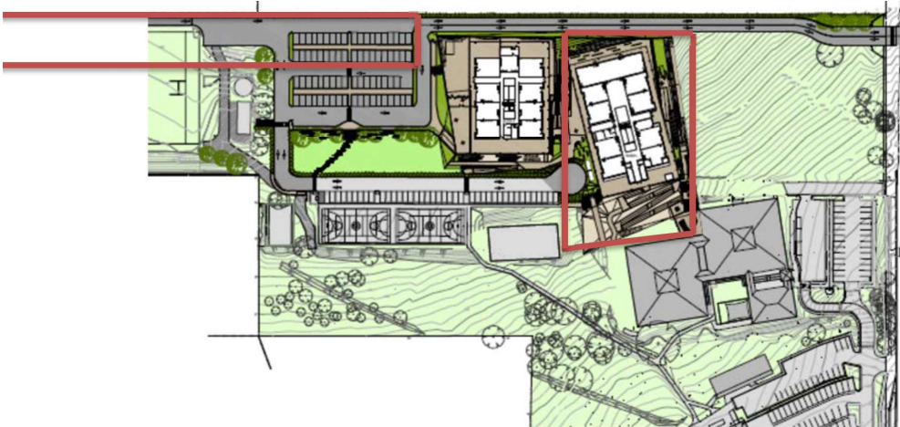
Figure 11 Stage 2: Construction of Junior Classrooms and second stage of car parking internal road network
