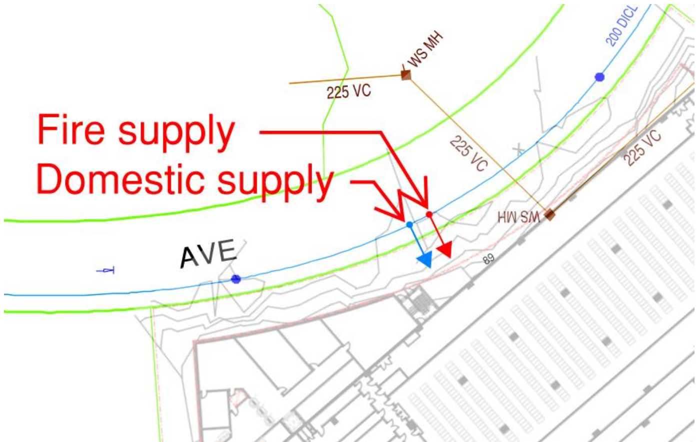
Figure 32: Water Supply Servicing Strategy
