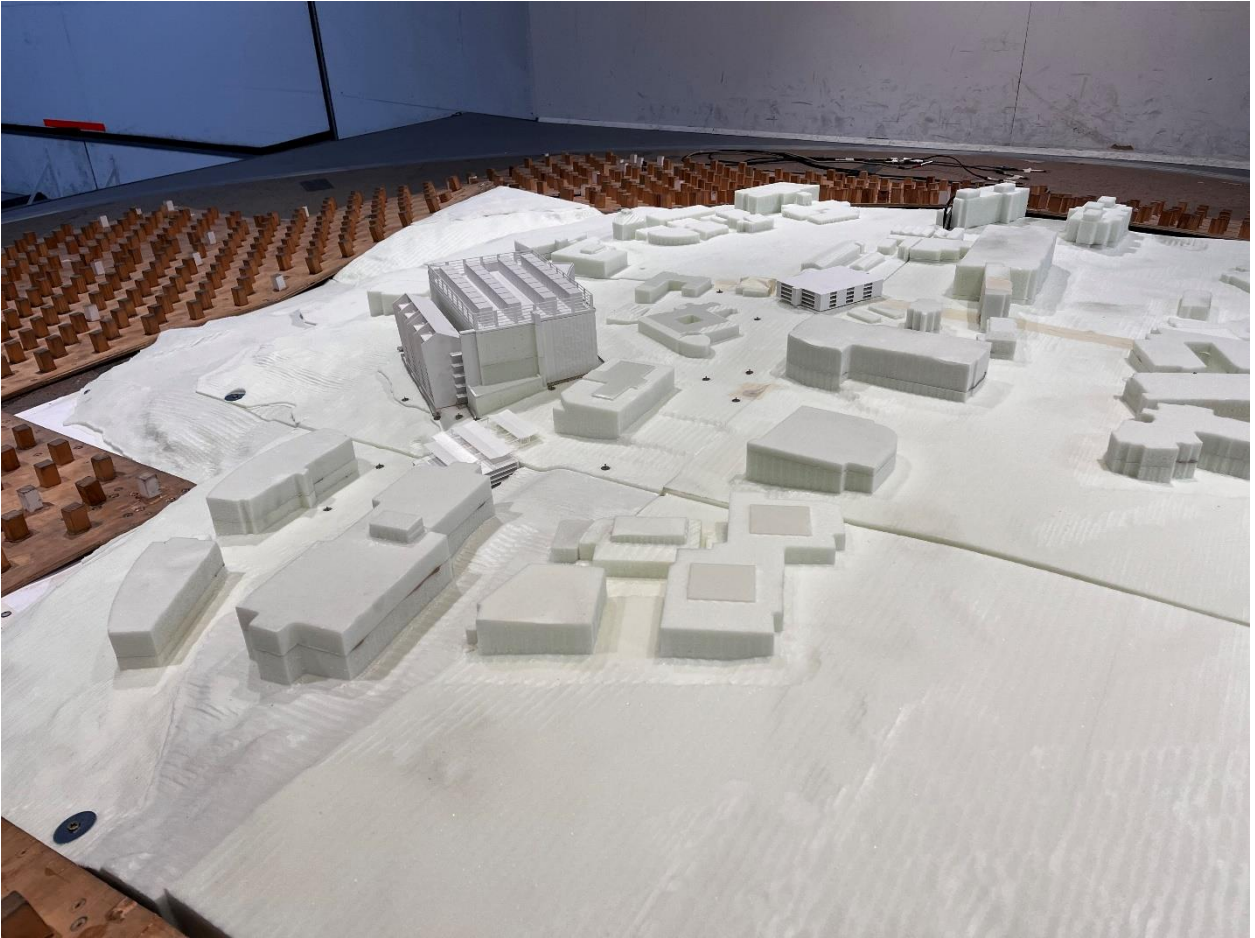
Figure 2d - View from the northeast of the 1/400 scale model of the proposed Julius Avenue Data Centre in the wind tunnel.
