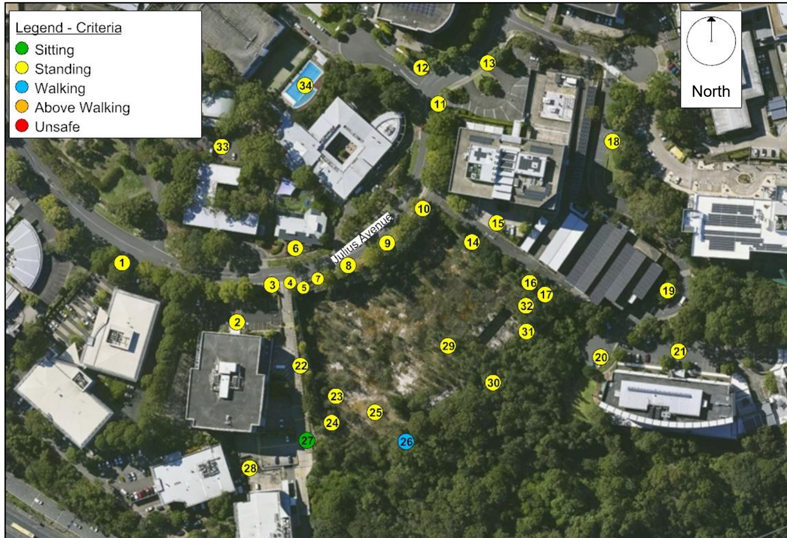
Figure 4 - Summary of wind criteria satisfied in the surrounding streetscapes for the Existing Configuration of the Julius Avenue Data Centre development.
