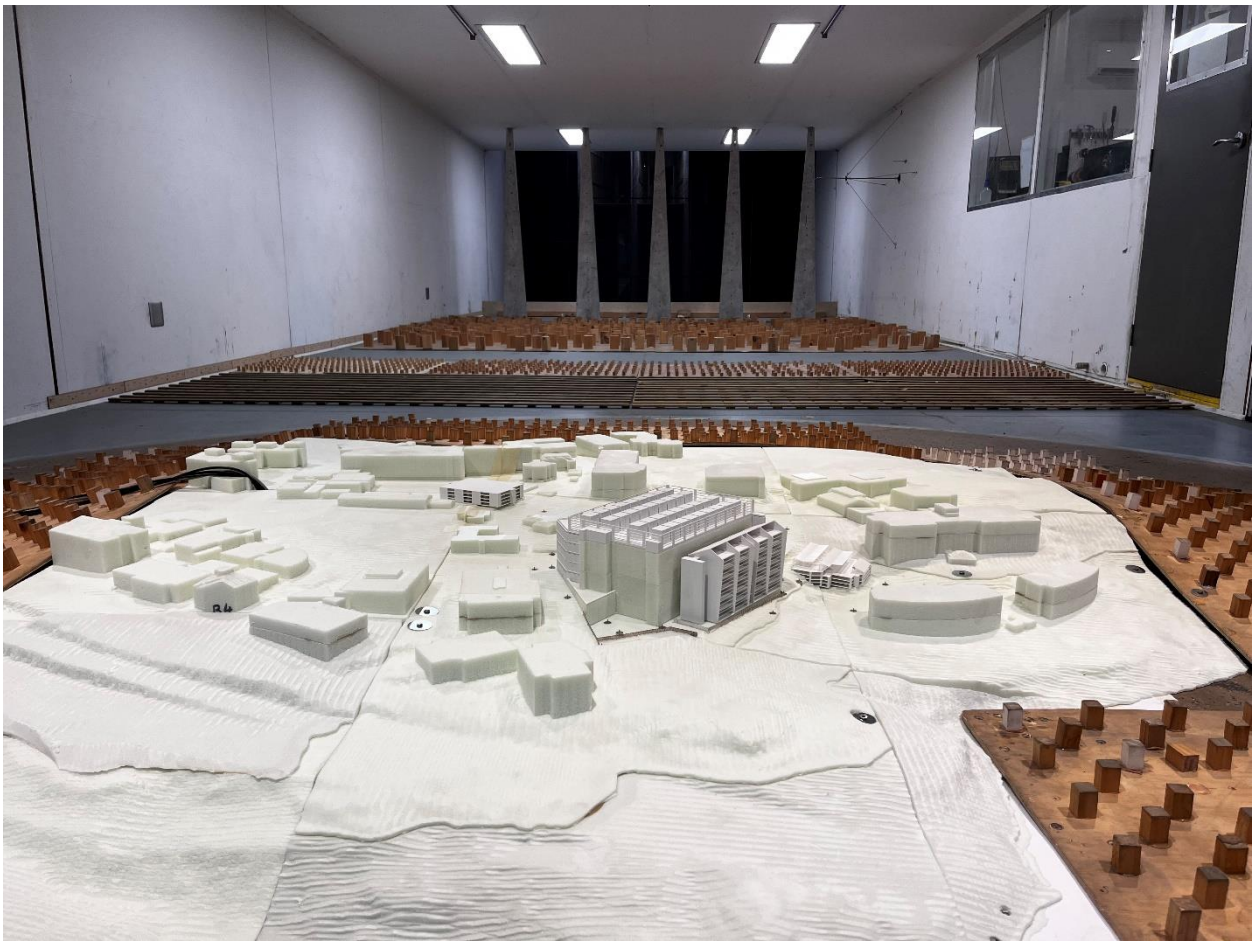
Figure 2a - View from the south of the 1/400 scale model of the proposed Julius Avenue Data Centre development in the wind tunnel.
