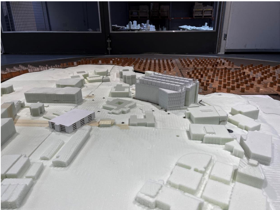
Figure 2c - View from the west of the 1/400 scale model of the proposed Julius Avenue Data Centre development in the wind tunnel.
