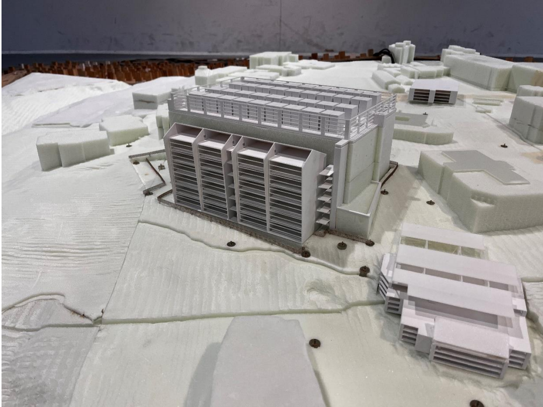
Figure 2b - Close-up view from the east of the 1/400 scale model of the Julius Avenue Data Centre development in the wind tunnel.
