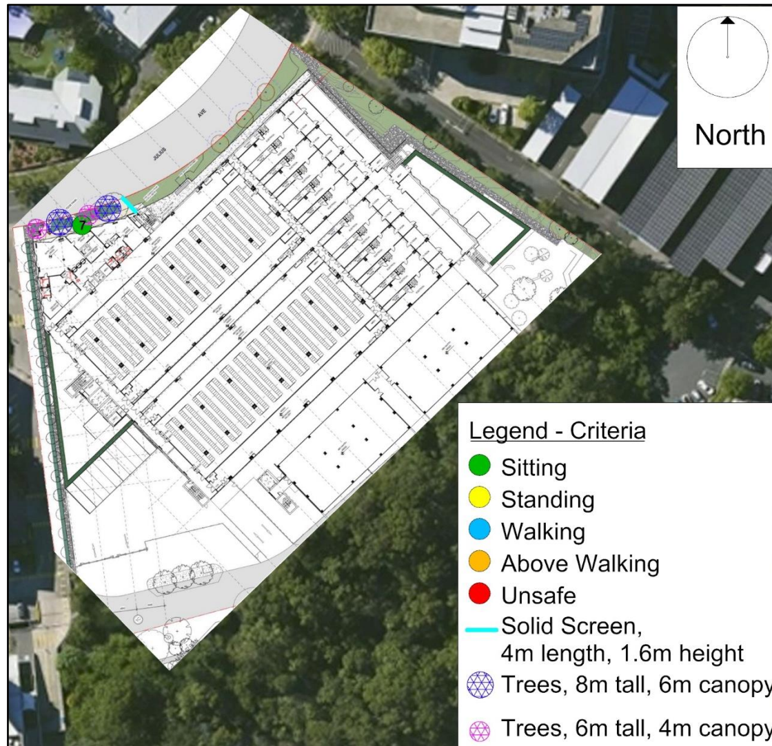
Figure 6 - Summary of wind criteria satisfied for the Proposed Configuration with wind mitigation at the ground level seating area of the Julius Avenue Data Centre development.
