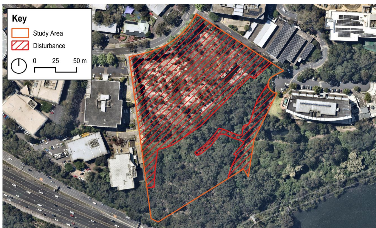
Figure 2.19 Map of areas of significant disturbance, ie deep excavation, construction of buildings, driveways or substantial land clearing for vehicle tracks. Note that minor areas of land clearing for pedestrian tracks have not been mapped as disturbance, as these impacts are likely to have been more minimal. (Source: Nearmap with GML overlay, 2025)
