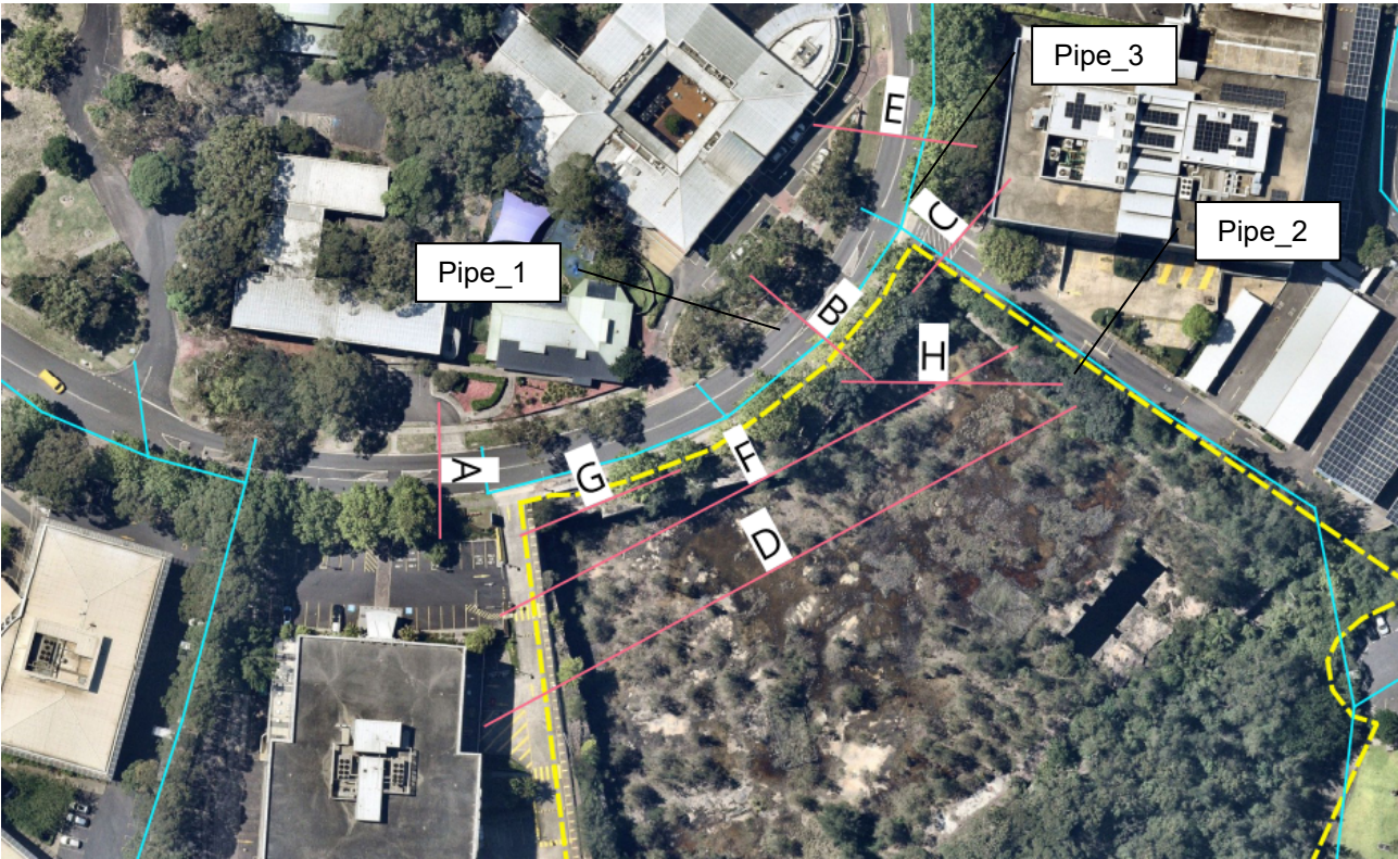
Figure 9- The location of PO lines and pipes from which the flow was extracted
