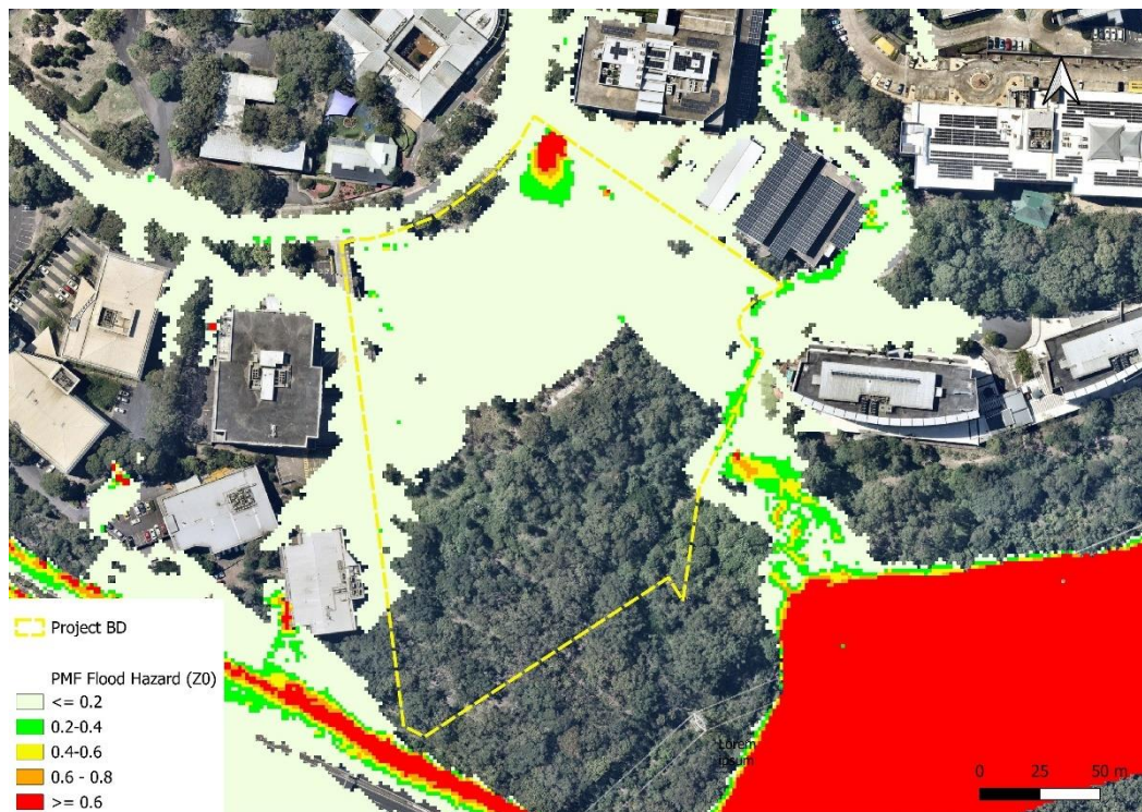
Figure 38- PMF Flood Hazard (Z0)- Existing Scenario
