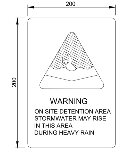
ON SITE DETENTION WARNING SIGN TO BE PROVIDED IN A VISIBLE LOCATION NEAR OR IN BASIN AREA
