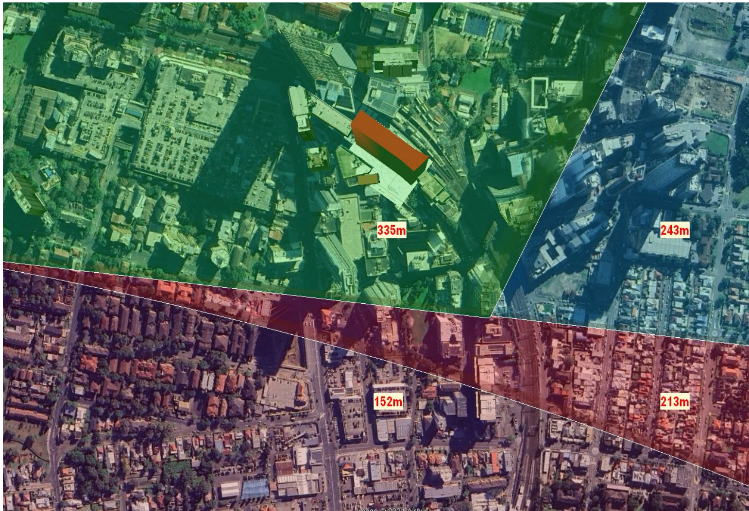
Figure 16: Avlaw model showing buildings below the RTCC over the site showing built and temporary structures below surface
