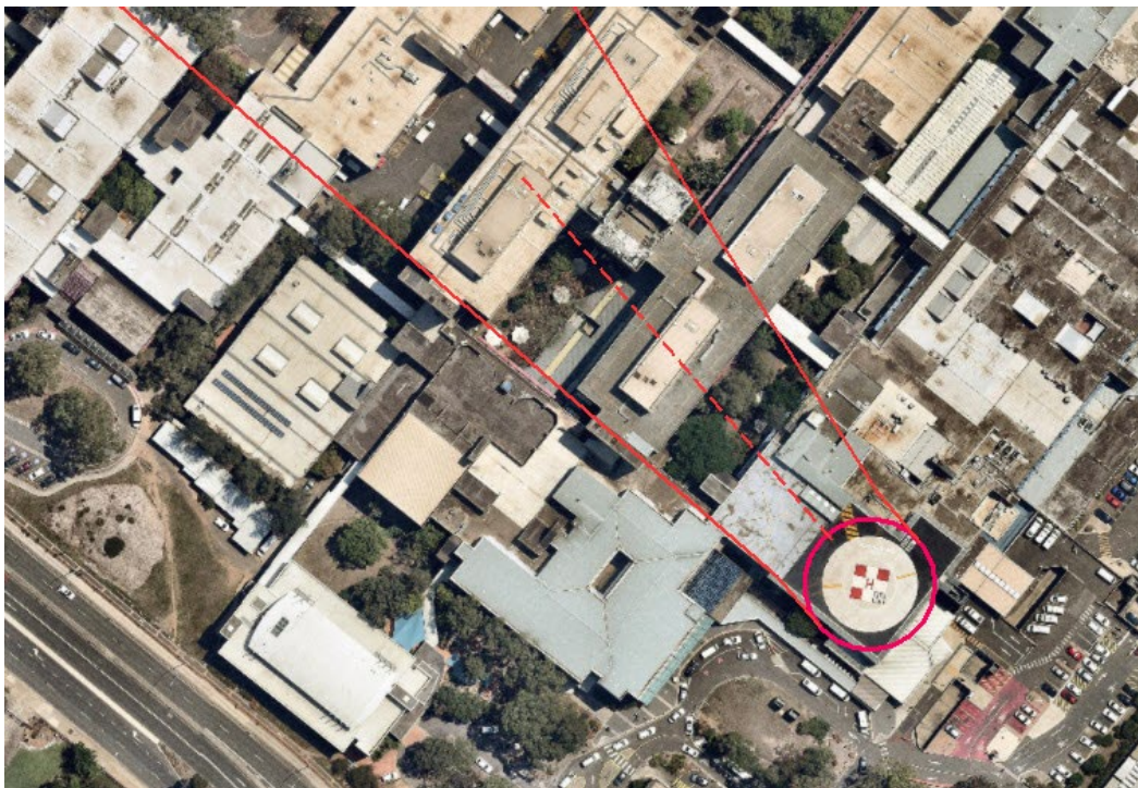
Figure 20: CASA AC139.R-01 v3.1 helipad operational airspace for RNP 127M flight path (A&E HLS)
