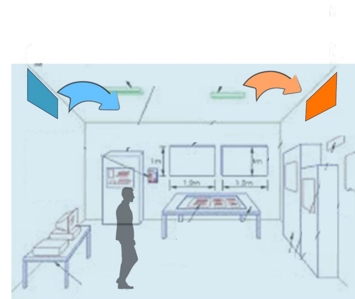
Example fire control room with large supply and exhaust grilles.
