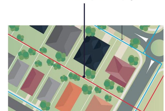
Example council sewer line running through a property.
