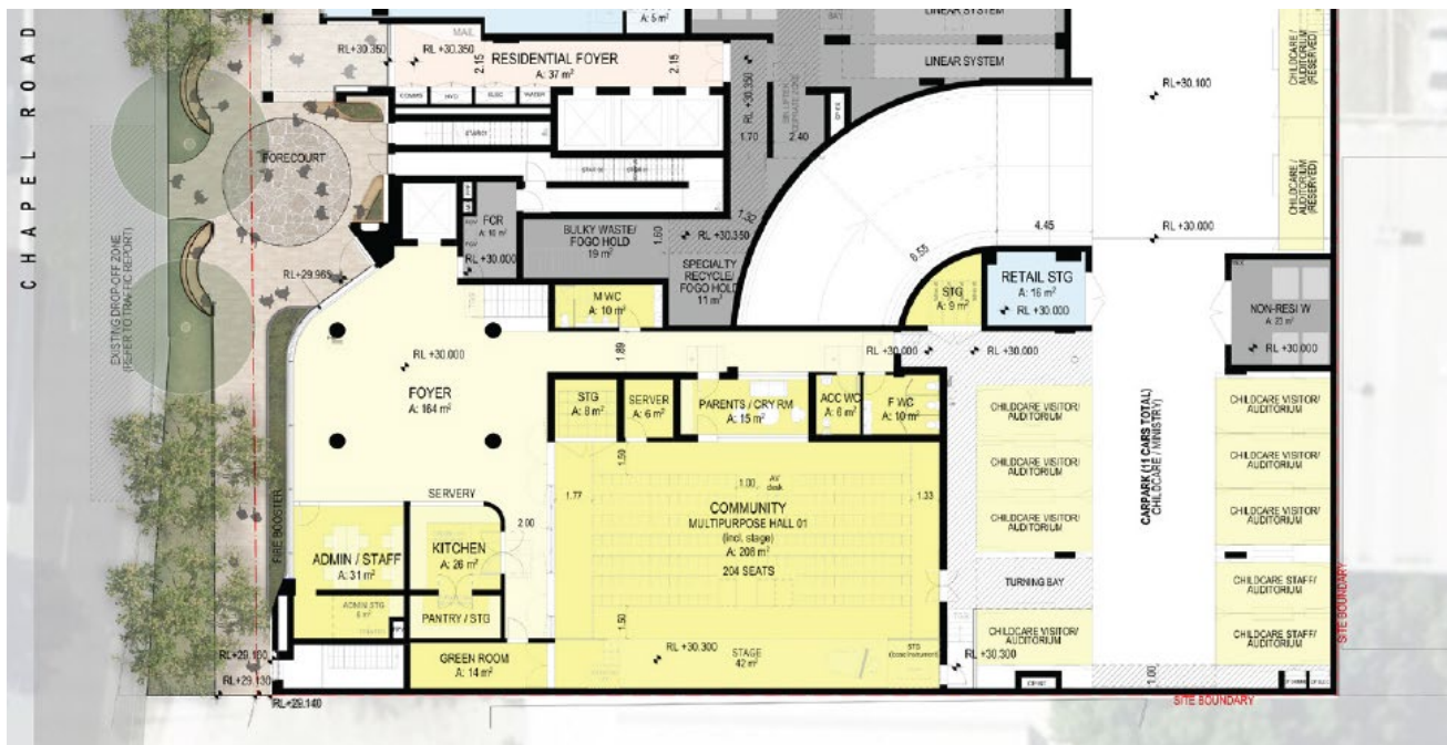
Figure 14 Floor plan of ground floor shared place of public worship and community facility
