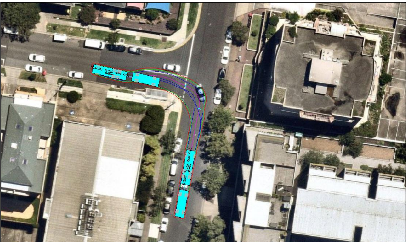
Truck and Dog Left Turn from Jacobs Street onto French Avenue Successful
