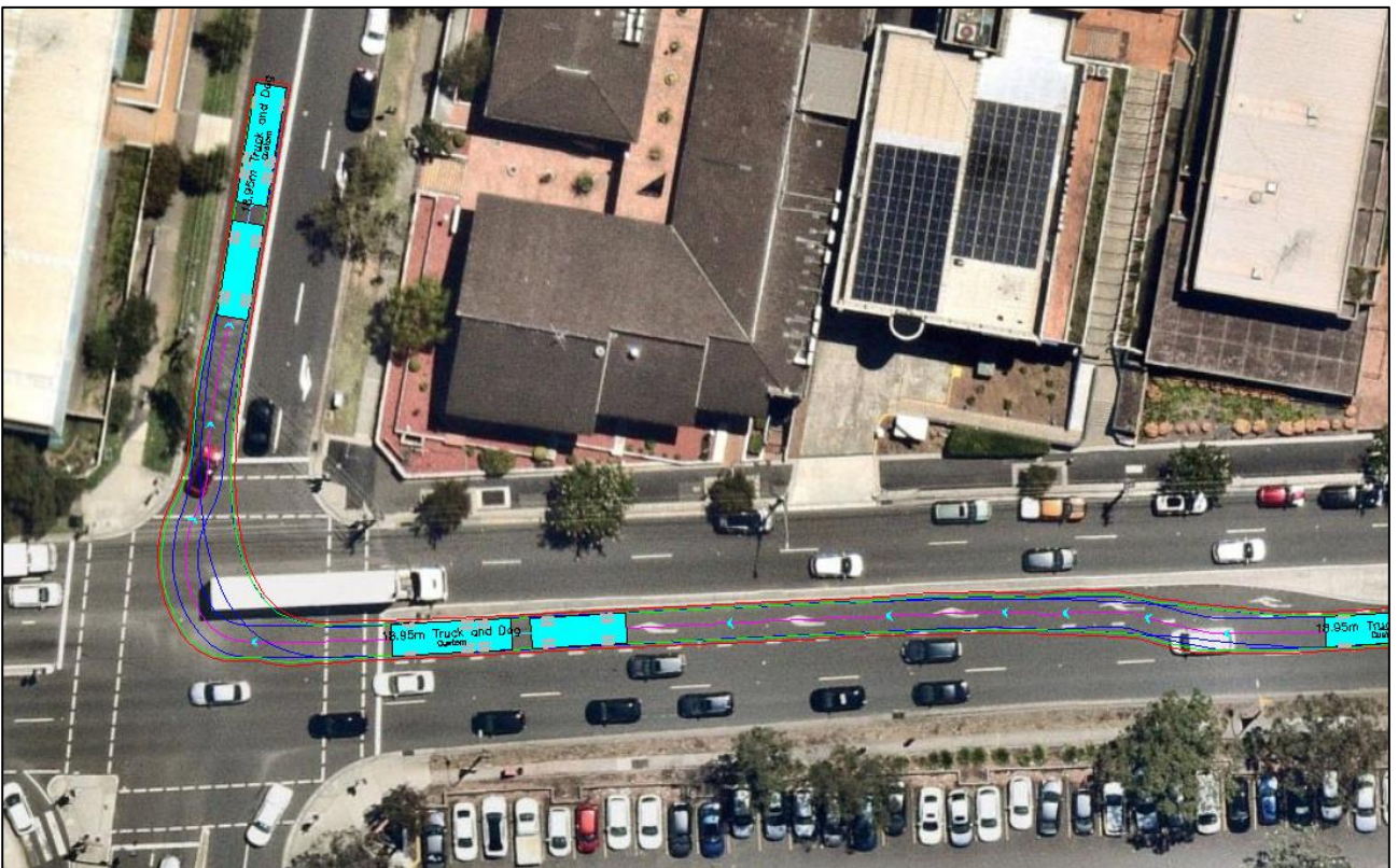
Truck and Dog Right Turn from Rickard Road onto Jacobs Street Successful
