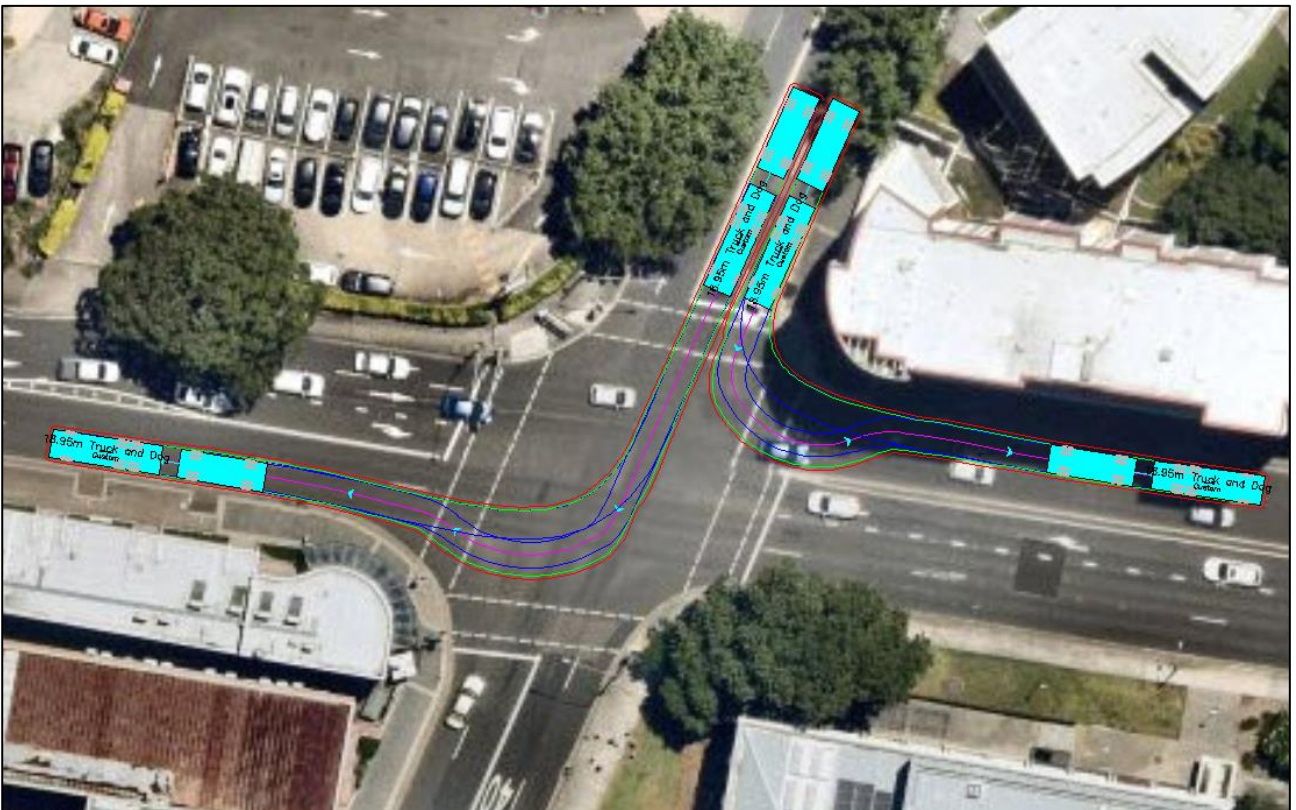
Truck and Dog Left and Right Turn from Chapel Road onto Rickard Road Successful
