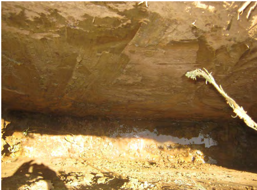
Photo 6 - Groundwater encountered at TP6
