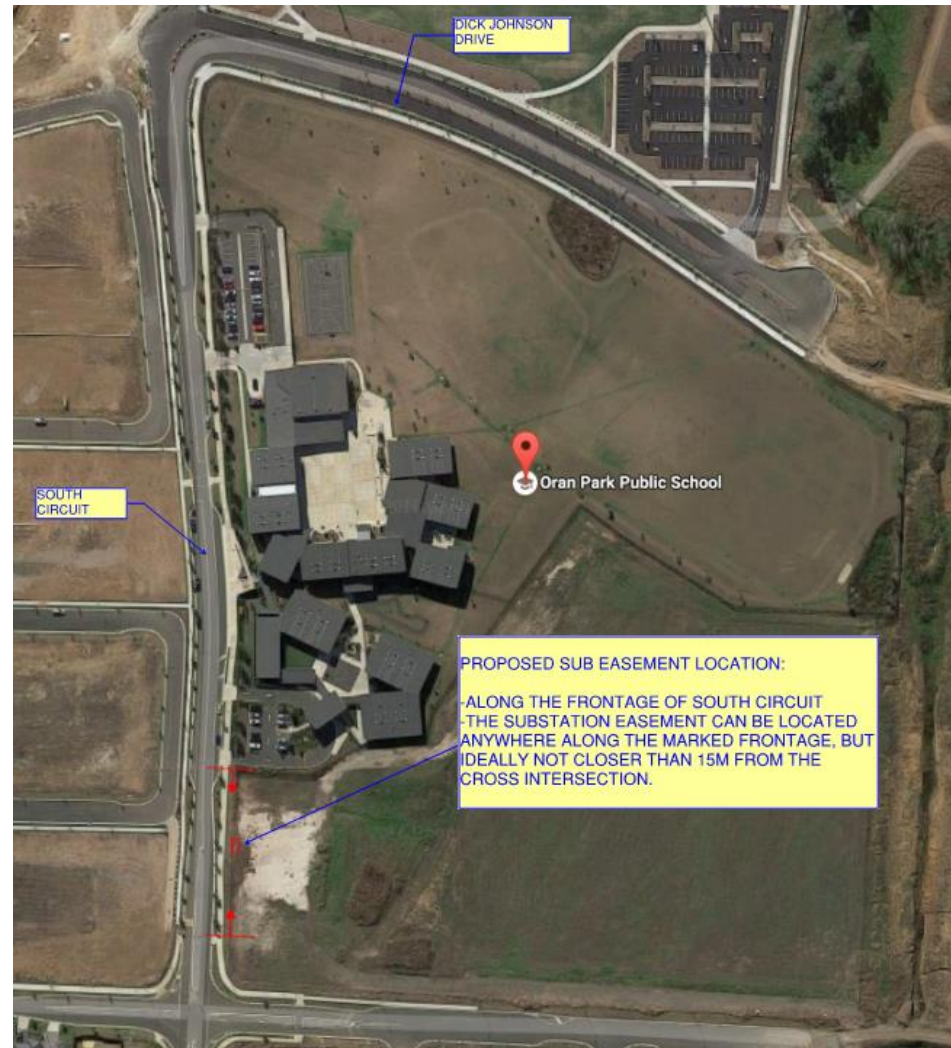
Figure 5 – Proposed Location of New substation.
