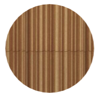
03. PODIUM CLADDING GROUND FLOOR FACADE CLADDING WITH GLAZED FLUTED TERRACOTTA PANELS IN DARK SANDSTONE FINISH
