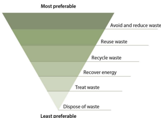
Figure – Waste Hierarchy - Reference: NSW EPA Waste Avoidance and Resource Recovery Strategy (2014 – 2021).
