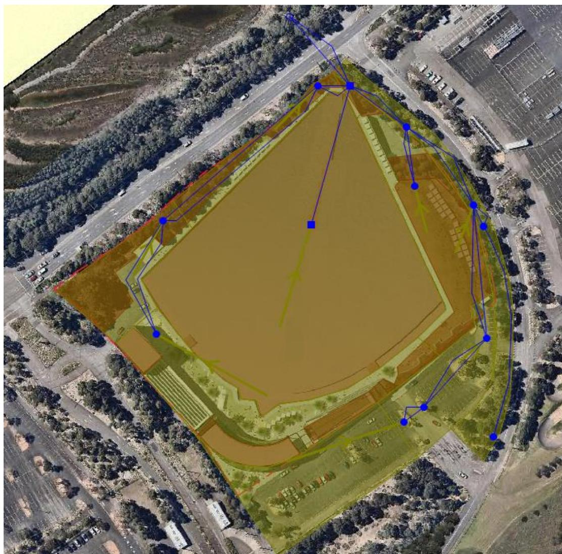
**Figure 7: Modelled post-development drainage system**
