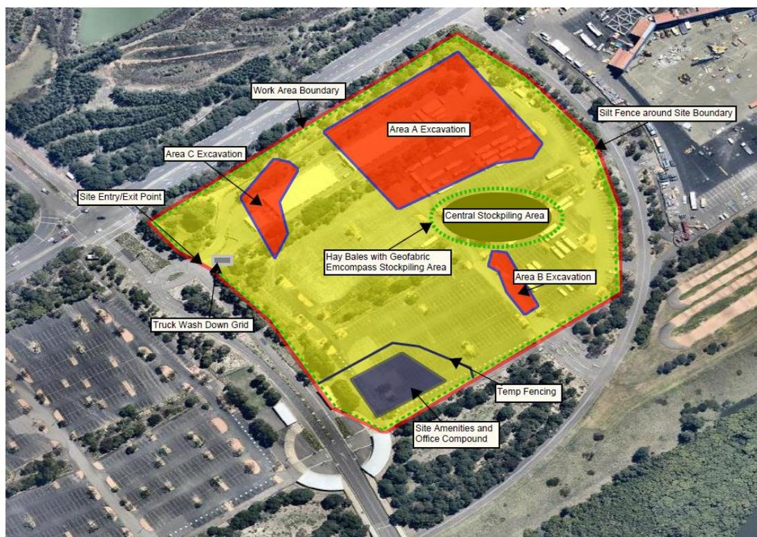
Figure 13: Sediment and Erosion Control Plan (Source: InSite Remediation Services)
