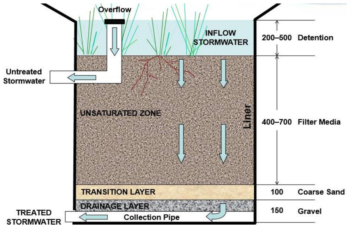
Figure 9: Typical bioretention area
