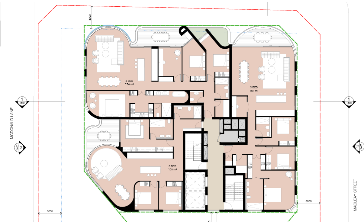
Figure 3 Architectural Plans – Levels 4-10 (typical residential floor plate)
