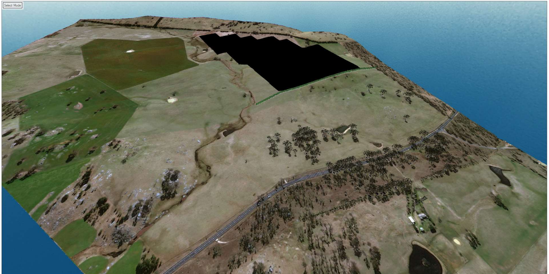
Figure 4 - Solar Array 200m setback. 4m tall.
