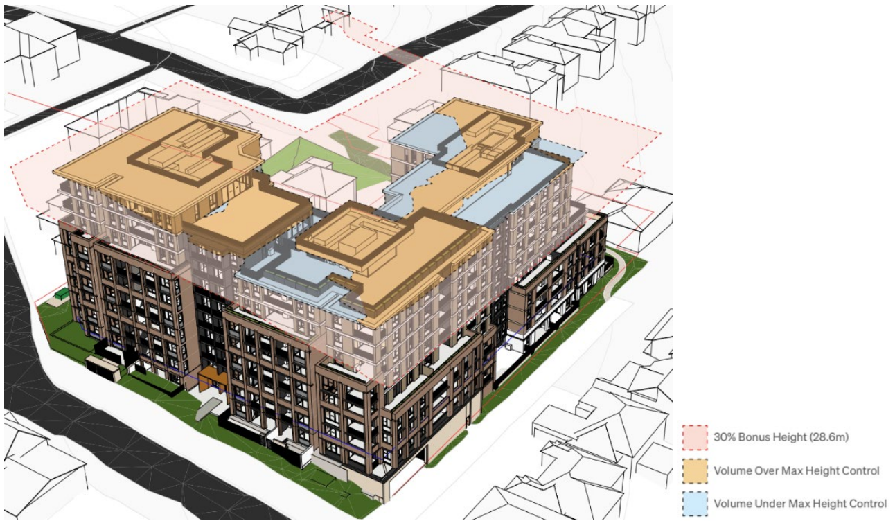
Figure 3: Building Height Plane – Volume over and under maximum height control Source: DKO
