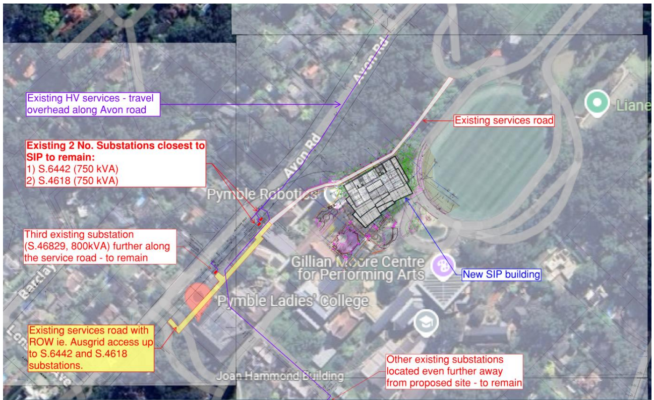
Figure 4 Site map of Existing substations and HV lines retrieved from BYDA and Ausgrid WebGIS data
